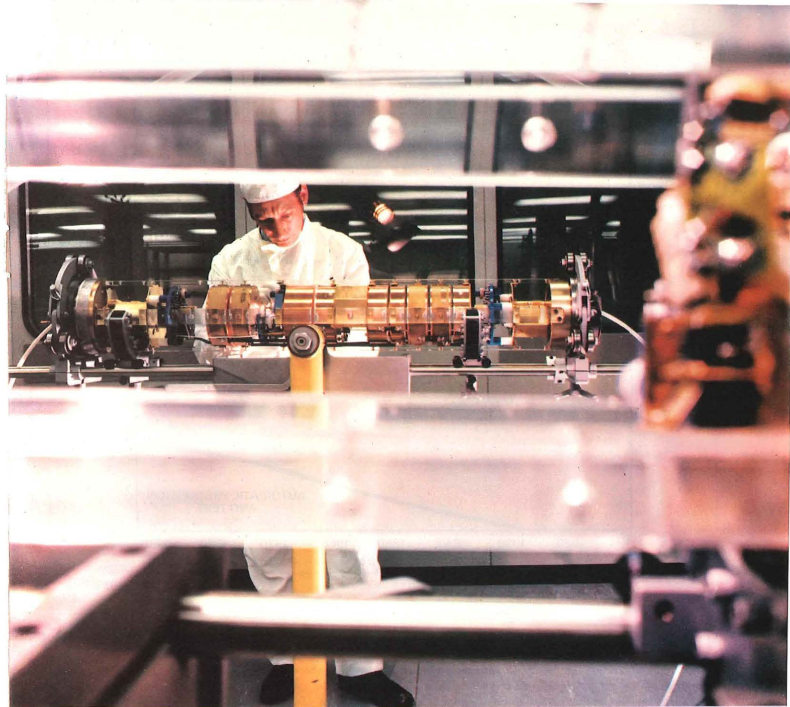
Repeaters for a modern, high-capacity undersea cable system are assembled at an STC factory.
