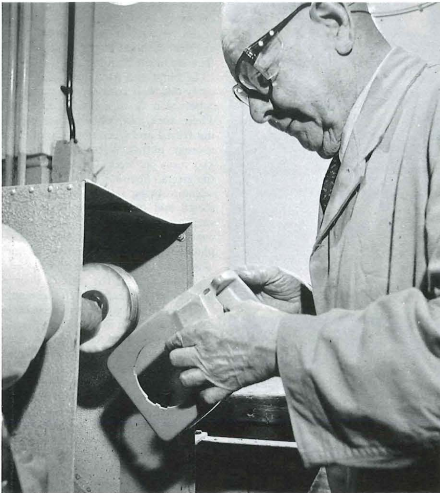
Ted Braidwood uses the buffer machine to polish up a telephone casing.
