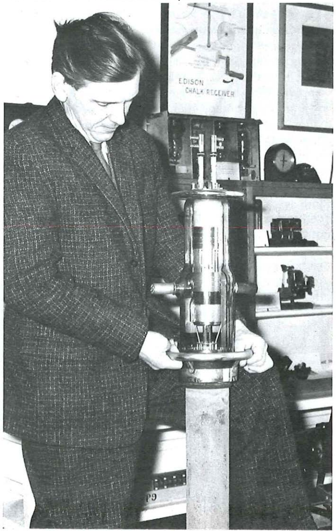
Below: Peter Povey holds a giant CAT10 water-cooled valve used on the first transatlantic telephone circuits in 1927.
