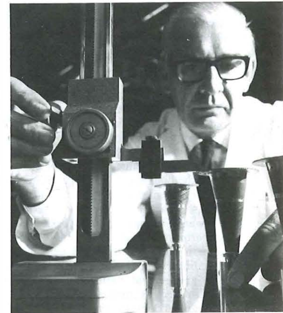
Below: A technician at the Research Centre measures an acoustic horn which will be used for testing transmitters in telephone handsets. Made of pure copper, each horn is produced by an electroforming technique to very close tolerances.
