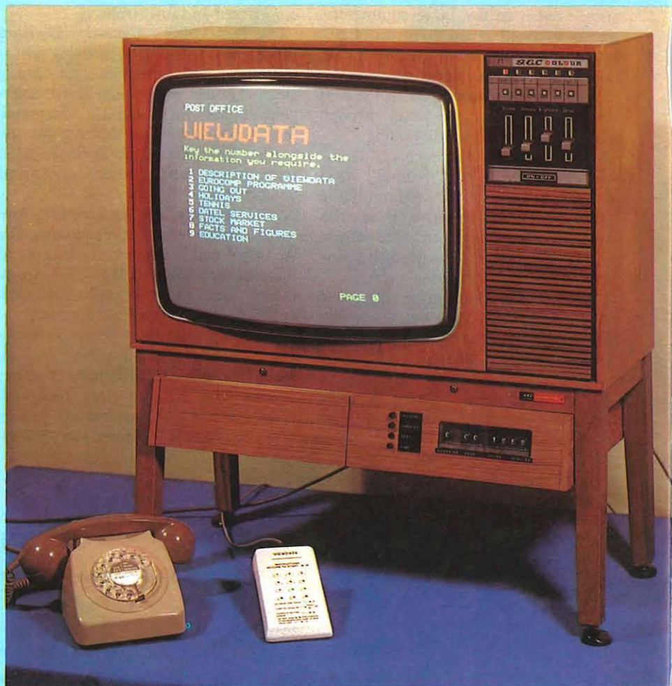
Basic equipment for a home user of the Viewdata service. Information can be displayed in up to seven colours.
