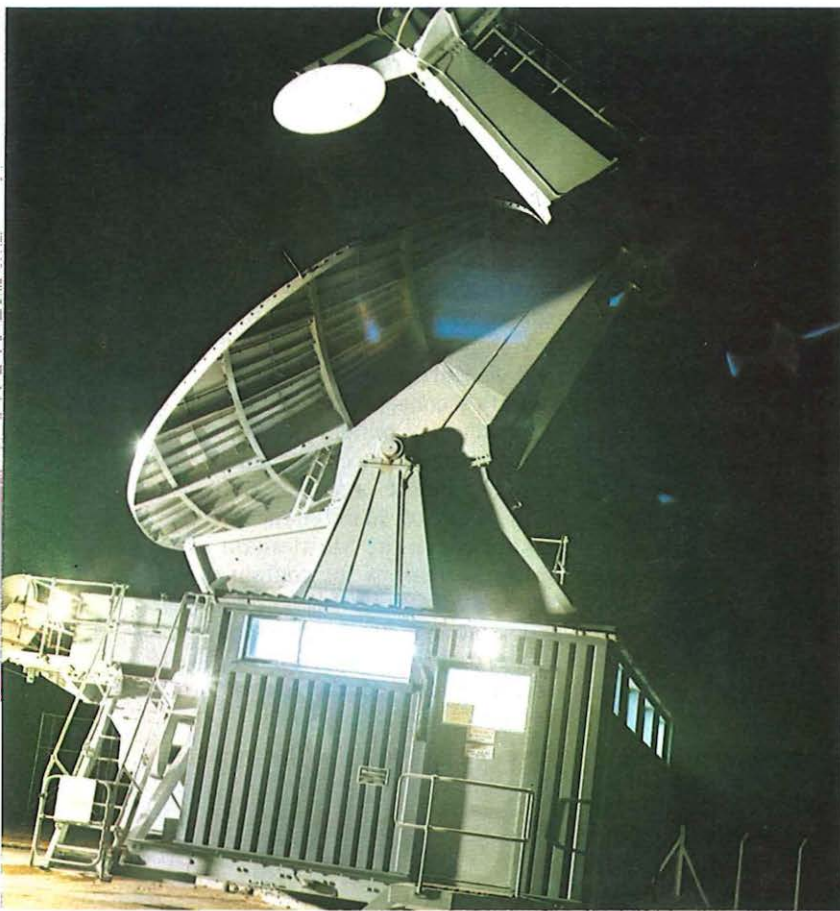
The 6-m diameter steerable aerial at Martlesham, which is used to obtain important data on the propagation characteristics of satellite-earth paths for future communications satellite systems.
