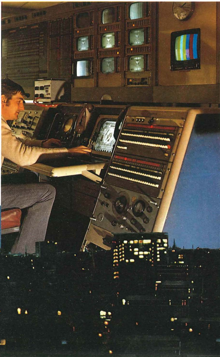
A Technical Officer at work in the Tower television control room where programmes from both home and overseas are switched.
