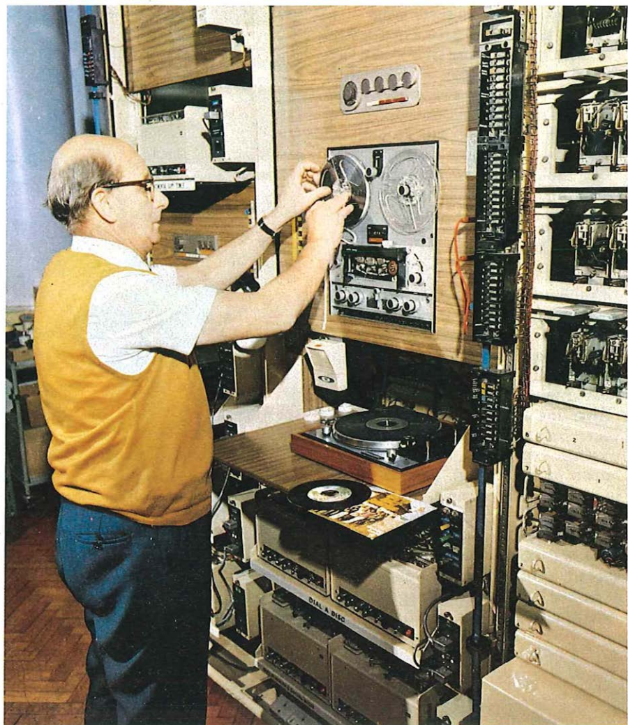
Below: Currently attracting more than 70 million calls a year is the dial-a-disc service. Here a recording is being transferred from an original disc on to tape, ready for use in the service.
