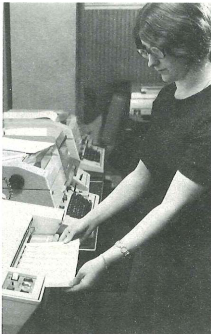
A transceiver is set up to transmit an urgent document from the THQ message relay centre to another facsimile machine within the Telecommunications Business.
