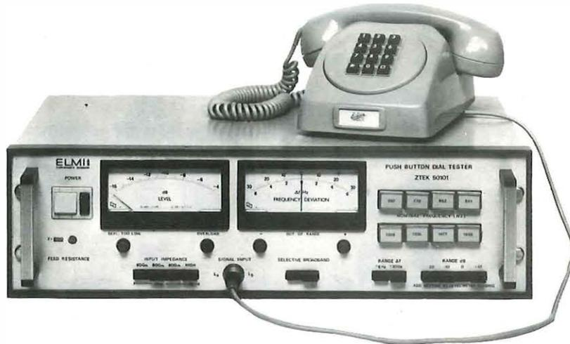
The ZTEK 50101 Push Button Dial Tester enables selective measurements of levels and frequency deviations to CCITT recommended frequencies used in Push-Button Telephone Sets.
