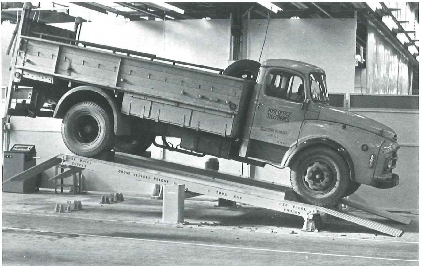
**One of the latest aids to vehicle maintenance is this lift which tilts to give easy access underneath the front and rear of a vehicle.**
