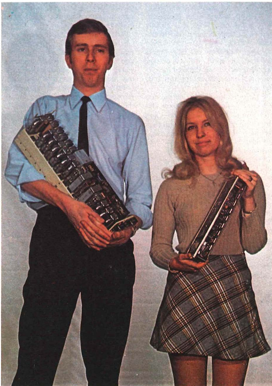
The extent of progress in the design of SSAC9 signalling equipment is clearly shown by this comparison of a new miniaturised unit, right, with an earlier type.
