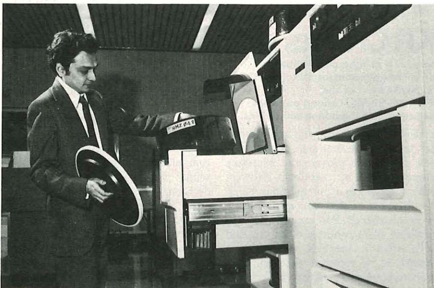
A powerful IBM computer recently put into operation by the Post Office can serve about 600 terminals. Here a user's file of data is loaded into the computer's disc file.
