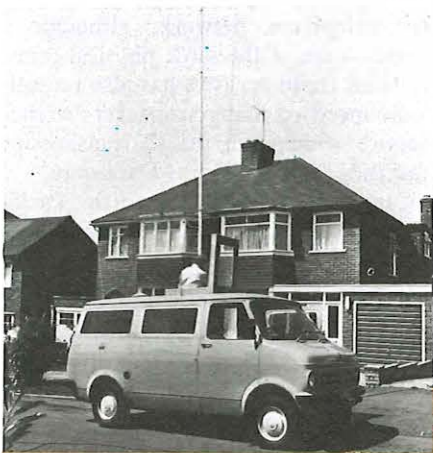
Left: The prototype vehicle incorporates a pneumatically-operated mast which can be extended to a height of 25 ft. It enables the operator to check television reception without using the complainant's aerial.
