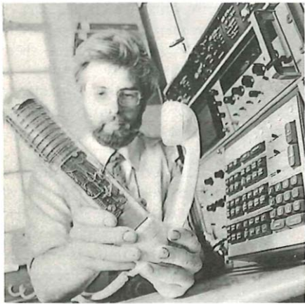
A Post Office research engineer in the transmission standards laboratory at Dollis Hill carries out sensitivity measurements on a telephone handset microphone. He is using a recently developed instrument which simulates speech, and measurements are processed by the computer seen in the background.
