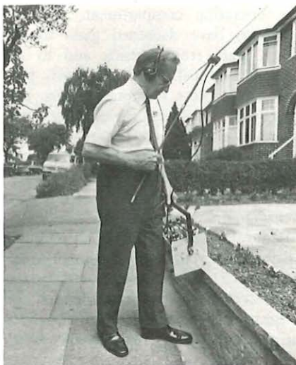
Portable receiving equipment is used to trace the source of television interference. The operator uses headphones while monitoring the broadcast to avoid causing a nuisance in the street.
