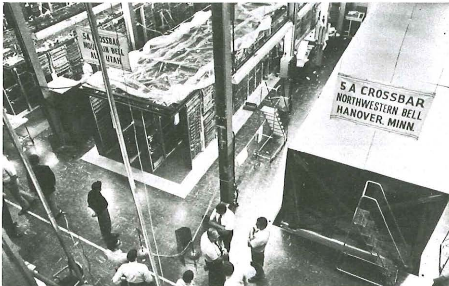
Crossbar 5A - mobile and modular telephone exchange units - are built, tested and packaged for delivery on specially designed lorry-trailer bays. When completed each unit is picked up by a lorry cab for transportation to its site.
