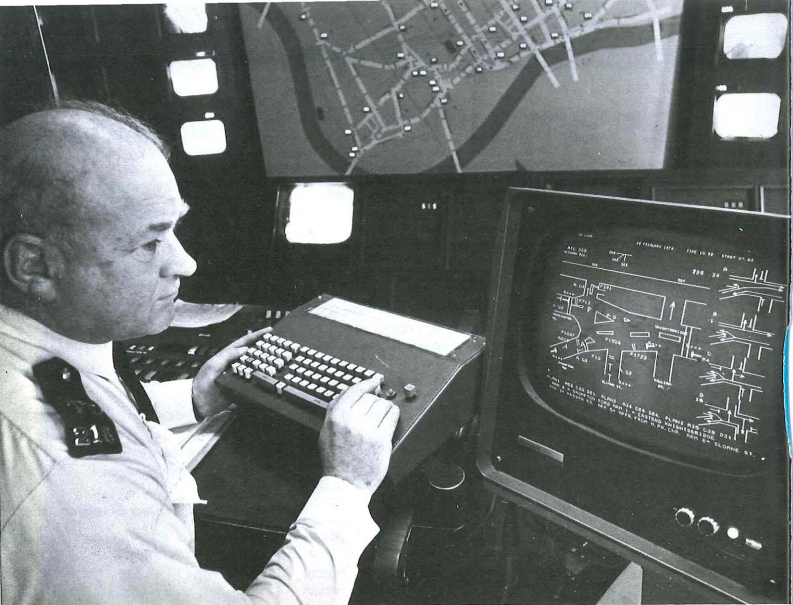
In the West London road traffic control centre at New Scotland Yard a police operator calls up the computer visual display of traffic light operation at a busy junction. In the background is a map of the area controlled by the scheme and television screens which show the state of traffic movement at the most important intersections in the area.
