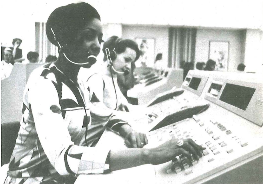
Computer-controlled Traffic Service Position Systems (TSPS) in the USA help to speed the connection of calls needing operator intervention. The equipment handles most routine details of setting up and recording calls, and very little work is required by the operators, who use simple push-button consoles.
