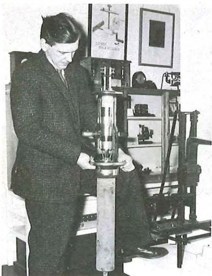
The curator holds a CAT 10 water-cooled valve of the type used in the first transatlantic cable in 1927. These huge valves required 14 gallons of distilled water a minute for cooling purposes.
