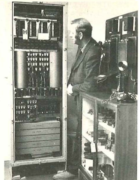
Calls can be dialled to this UAX 5, a complete 25-line automatic exchange of 1929, from typical installations of the period seen on the right.
