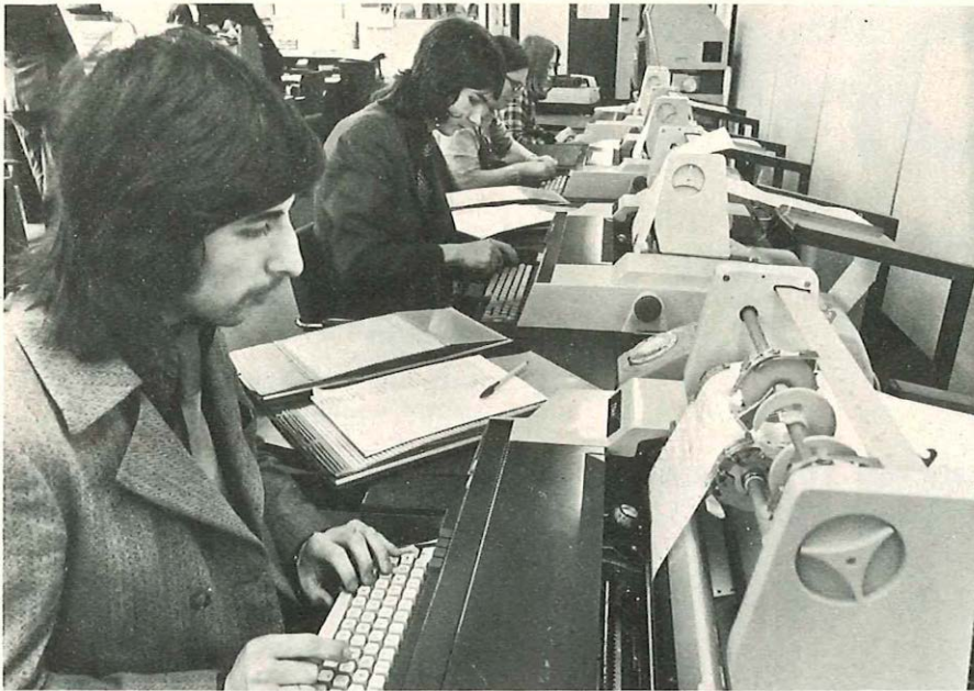
At the nerve centre of the network controlled from Woolgate House staff deal with transmission problems. Teleprinter-type terminals in the control room are used to "converse" with the computer.
