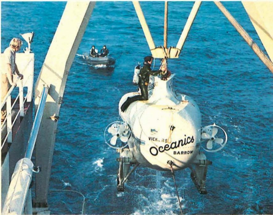
Above: The normal recovery operation when Pisces III was brought aboard her mother ship, Vickers Voyager, during earlier cable laying operations.
