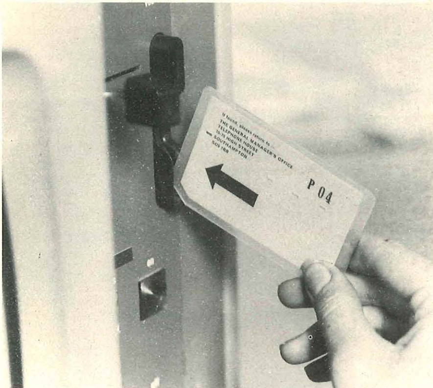
The security badge which must be inserted into a visual display unit before it can be operated. The badge identifies the operator.
