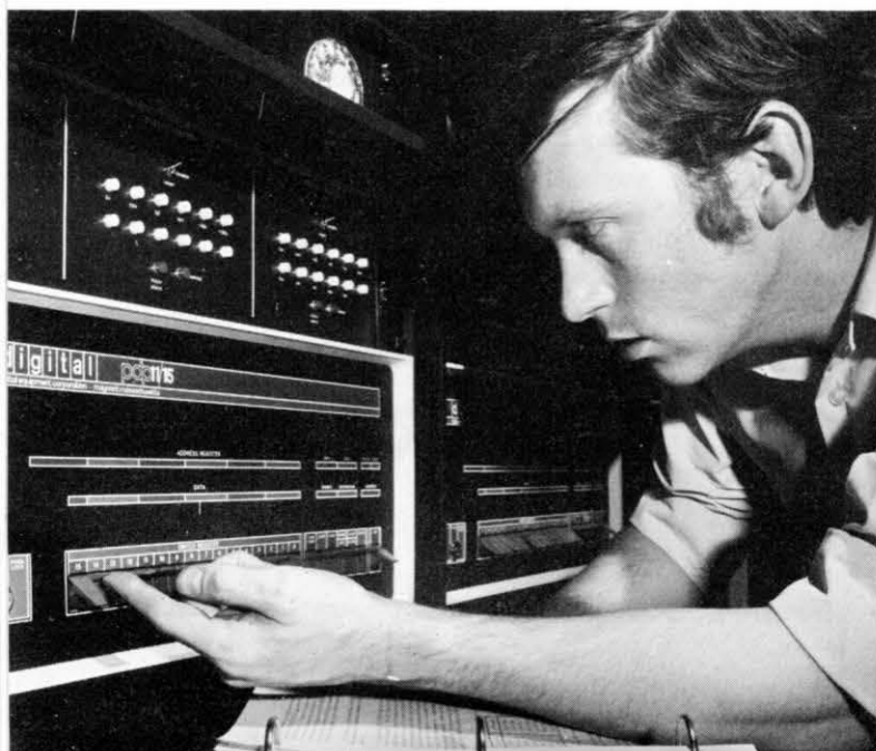
A Technical Officer at Reading Trunk Exchange programs the Radiopaging computer. It is done simply by selecting the appropriate switches on the front of the computer equipment drawer.
