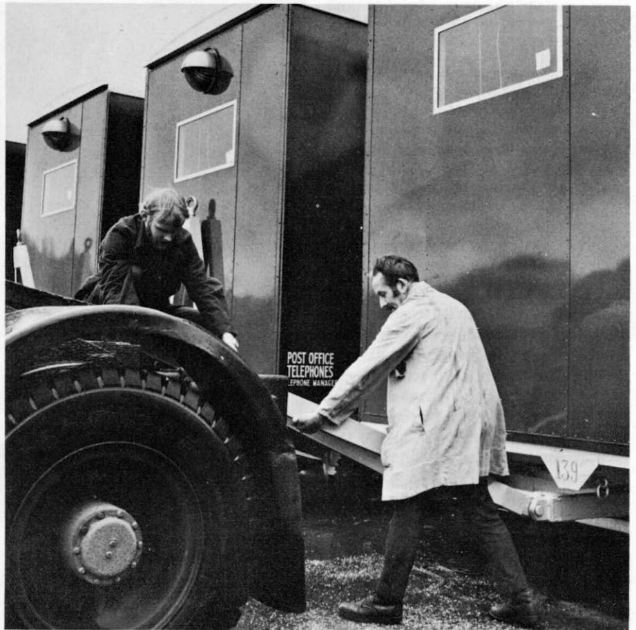
A mobile telephone exchange is hitched to the vehicle which will take it to an area where extra exchange lines are urgently needed. It is one of a new fleet of mobile exchanges which are being distributed throughout the country. See "A world first".
