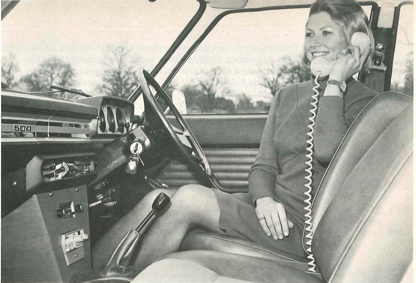
Above: The Radiophone control unit can be fitted into the dashboard or, as in this car, below a normal car radio in a console built over the transmission tunnel. The two knobs on the right of the unit are for channel selection and volume control. Two push-buttons on the left are for on-off switching and for calling the Radiophone exchange.
