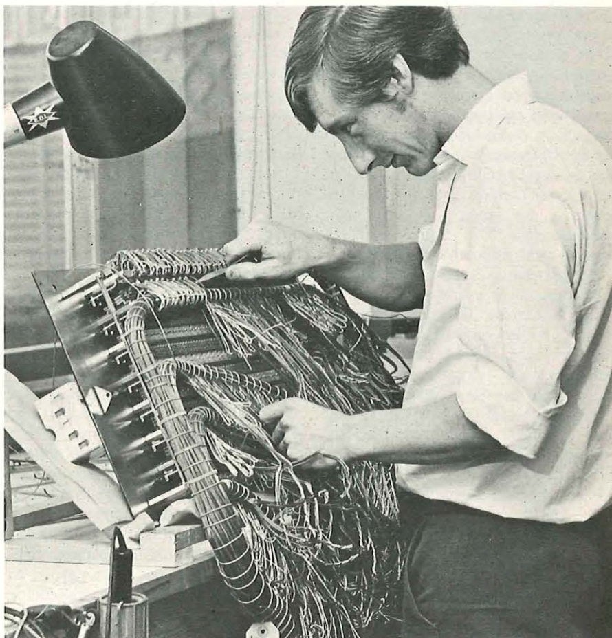
Technician Terry Smith at work on one of the 288-line key and lamp units later installed at the ambulance centre. All the units were wired and built at the South Central Telephone Area's workshop.
