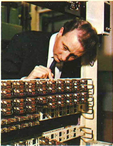
Above: Dave Locke, an Assistant Executive Engineer, examines the miniature relays which are reducing call-queueing problems. These little electronic devices "sense" a build-up of waiting calls and switch them to a free route much more quickly than before.
