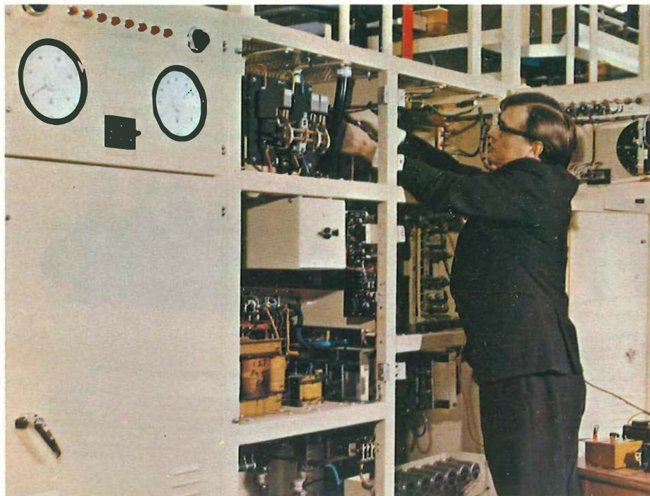
Executive Engineer Steve Humphreys, who has been responsible for much of the design work on the dc power modules, measures voltages during performance tests on the new equipment at the Telecommunications Development Department's laboratory in North London.
