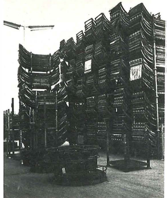
Below: Jointers' tents, stacked in the yards at the Crayford depot, await dispatch to the factory for repair.
