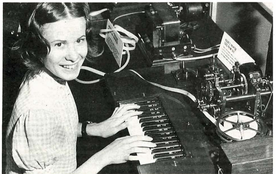
A visitor to the telegraph exhibition tries the piano-like keyboard of the Hughe's printer, in use from 1867 until as late as 1939.
