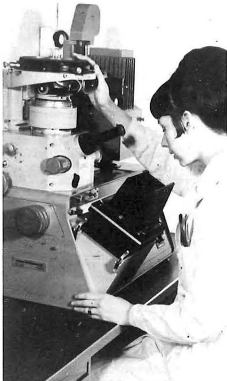
In the Birmingham Materials Section laboratory a projection microscope is used to examine metals.
