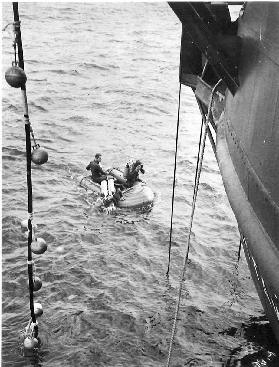
Skin divers about to go overboard from their rubber dinghy to disengage the seaplough from its davits. On the left is the vital control cable which carries signals and power between the plough and the towing vessel. The floats attached to the cable keep it above the plough.
