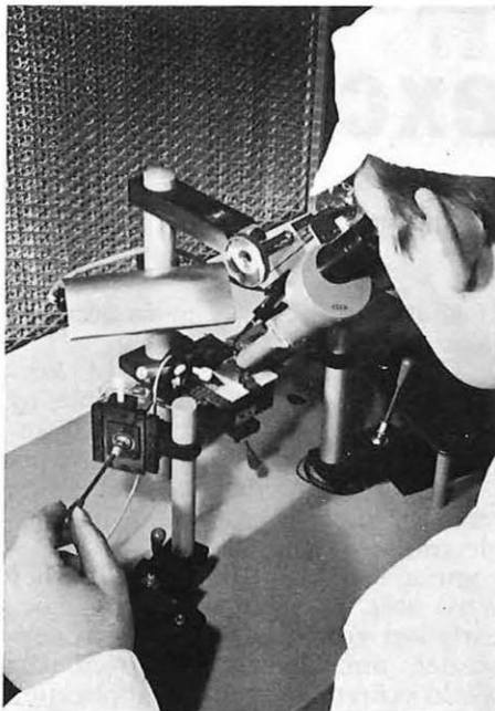
A minute MOST wafer is tested by an engineer in the Clean Room Laboratory of the TMC Company at Dulwich.
