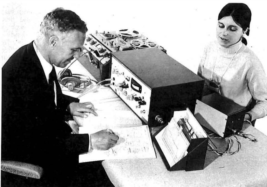
The author examines a "patient" who has a hearing-aid with the new STS equipment. On the "patient's" left hand is the volume control which she can adjust to hear the spoken word or tape recordings more clearly. In the centre is the master control unit which records the frequency response.
