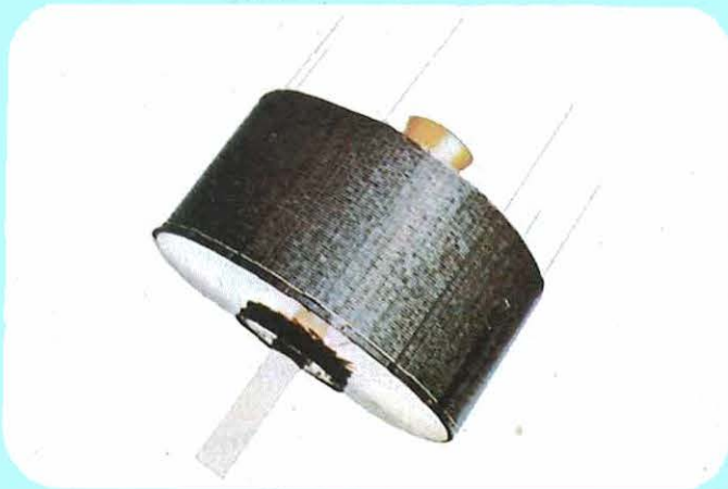
INTELSAT II—1967 Coverage: Atlantic and Pacific basins Diameter: 56 inches Solar drum height: 26.5 inches Weight: 357 lb at lift-off 192 lb in orbit
