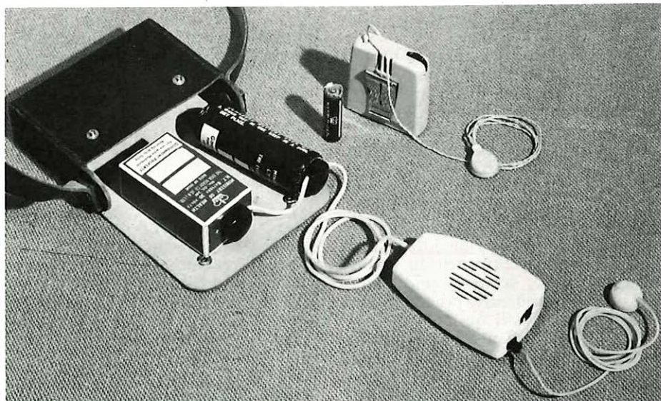
In the foreground is one of the last aids to use electronic valves requiring large batteries. Beside it the small transistorised hearing-aid, with its battery, now in general use.
