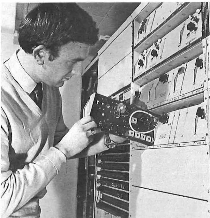
The first pictures to be published of the transistorised video equipment which the Post Office used to upgrade transmitter and studio links. Its big advantage over previous equipment is in its use of printed circuit cards. When a fault occurs the card can be removed, replaced immediately by a stand-by, and the faulty card repaired on the bench. As a result the transistorised installation need never be out of service
