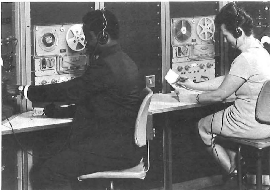
The measuring console, staffed by Mrs. Phyllis Redmond and Mr. Richard Oduraiya, which provides facilities for tape recording and speech voltage measurement.
