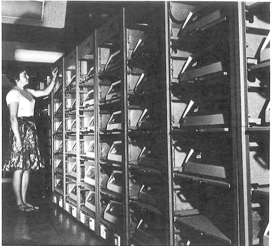
This computer bureau uses Datel 200 and offers time-sharing facilities for firms who want problems solved by computer. A number of modems No. 2 are rack mounted.
