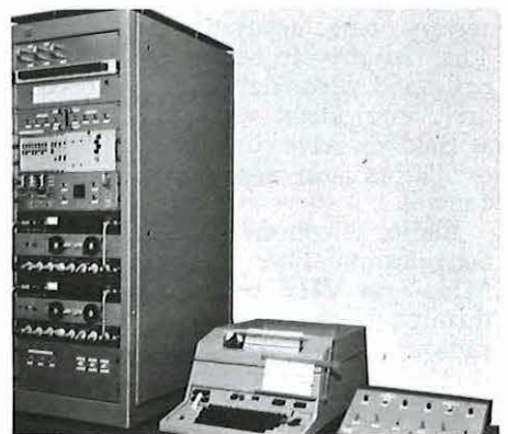
Below: Post Office equipment used on board the ship. From the left— dual diversity radio receivers and error correcting telegraph equipment and a Teleprinter No. 15 A, the latest development in teleprinters, used for the first time on board a ship, with its associated control box.
