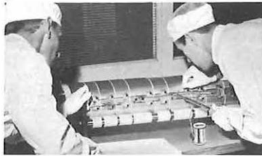
Ersin Multicore Solder is shown being used at the Erith factory of Submarine Cables Ltd., in the production of a submersible repeater designed to last for a minimum of 20 years under the sea without attention.
