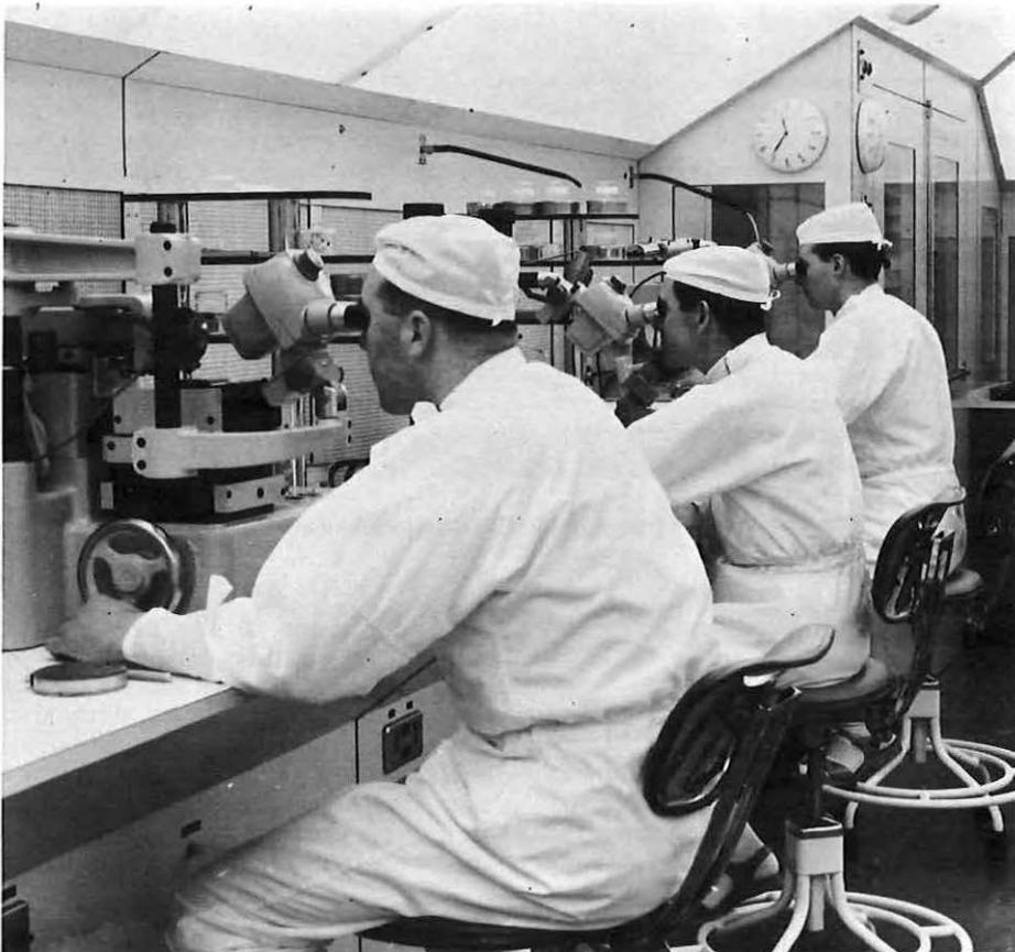
Staff wearing special caps and clothing assemble the transistors in the super-clean laboratory at Dollis Hill.
