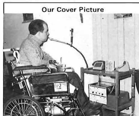
Our Cover Picture A patient at Stoke Mandeville Hospital operating the puff suck telephone.
