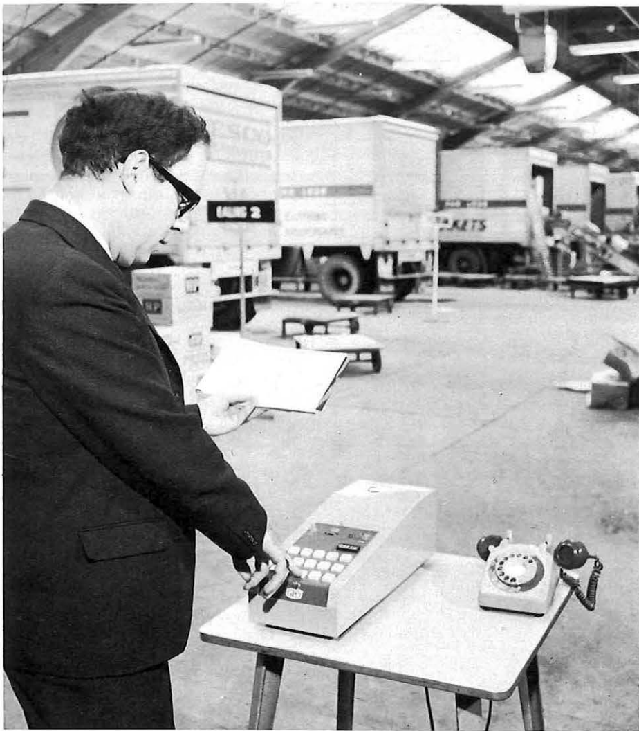
This is a Datel 300 outstation at Tesco House providing touch-of-a-button information for the efficient operation of Tesco stores and transport.
