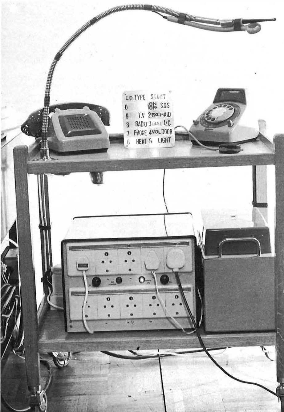
The equipment required for the LST 5B. In the centre on the top of the trolley is the visual display unit which shows the user the various stages of the operation.
