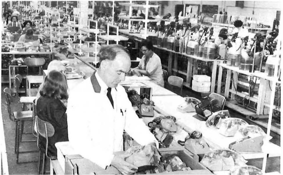
GPO telephones leaving the production line fully assembled and tested are wrapped in protective polythene film before being finally packaged and despatched.
