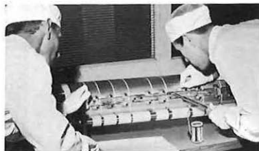
Ersin Multicore Solder is shown being used at the Erith factory of Submarine Cables Ltd., in the production of a submersible repeater designed to last for a minimum of 20 years under the sea without attention.
