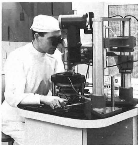
A technician at the Post Office's Dollis Hill Research Station at work in the controlled environment laboratory where the new long-life transistors are produced.
