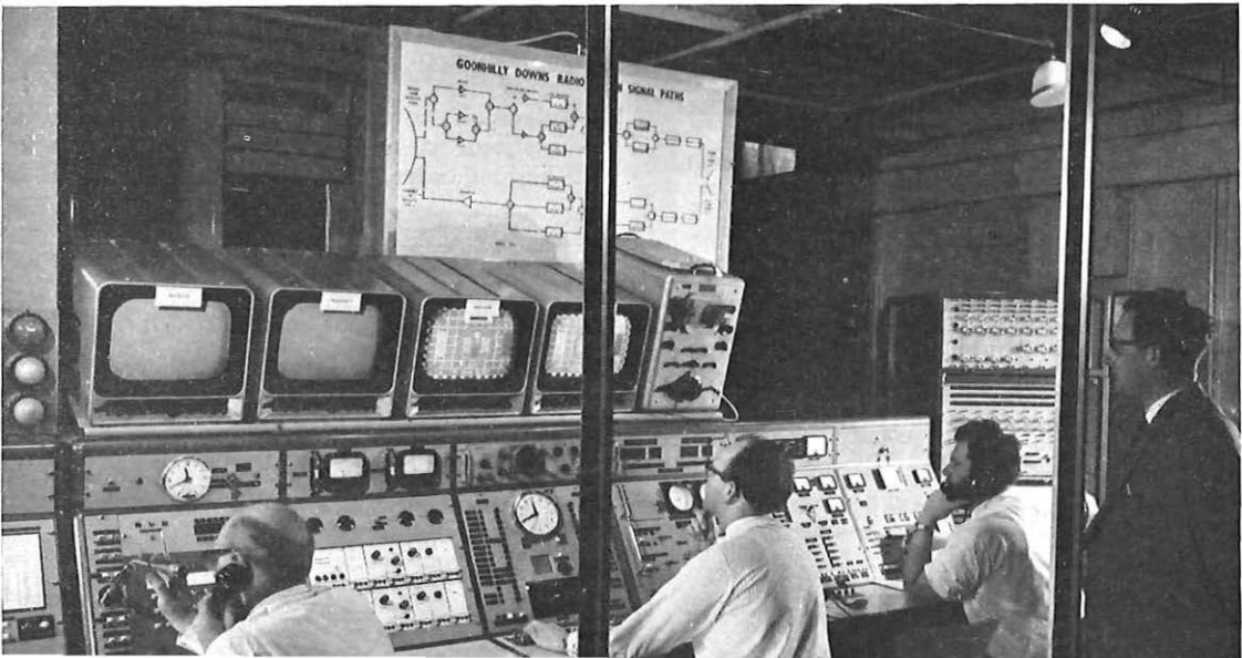
Below: Engineers monitoring satellite transmissions at the main operating console at Goonhilly. Right: Map shows the locations of the earth stations and satellites used for TV and radio coverage of the Games.
