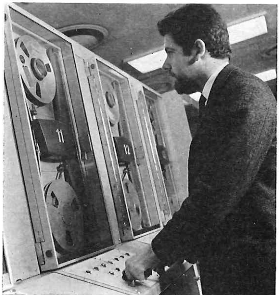
The Telecommunications business is going in for computerisation in a big way. Here, an operator at the London Computer Centre sets up the controls of a magnetic tape deck.
