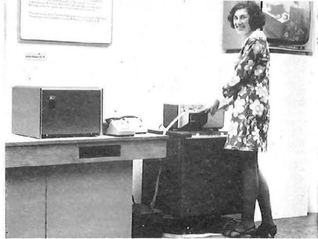
Left: Earl Mountbatten of Burma tries out the Datel 300 Service, one of those on display at the IFIP Congress in Edinburgh. Above: The Post Office Datel modem No. 7, for the new Datel 2,400 Service, working for the first time with the STC GH210 data terminal at 2,400 bits a second.
