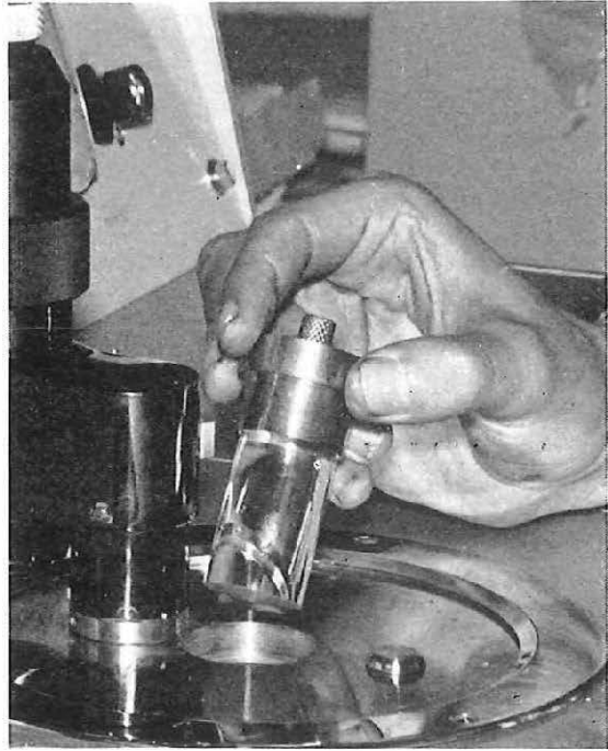
Above: A close-up view of the polished sample of optical glass. Below: The diagram shows the formation of the glass fibre cable. Each fibre, of which there would be several hundreds, would be able to carry thousands of times more information than a pair of copper wires in the present cables.
