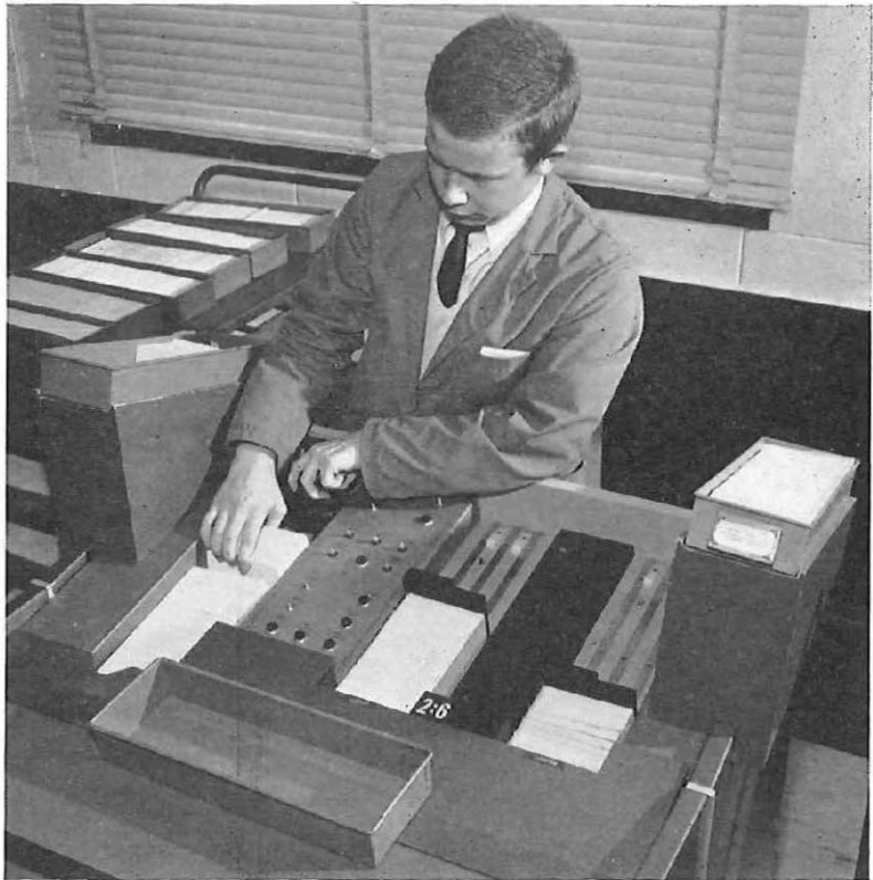
Machine Operator Roger Tutton at work on one of the 40-column card readers in the computer room.
