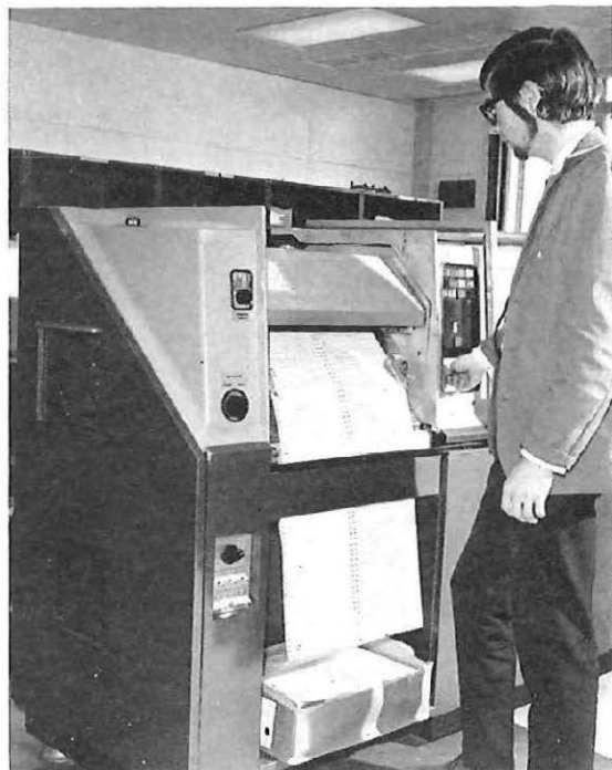
Left: 80-column cards holding information about payments, meter readings and advice notes are fed into a reader in the computer room. The Machine Operator is Graham Watts. Below: The Analex printer, operated by Antony Jolliffe, is used to print telephone bills, trunk statements, reminders, reports and listings.
