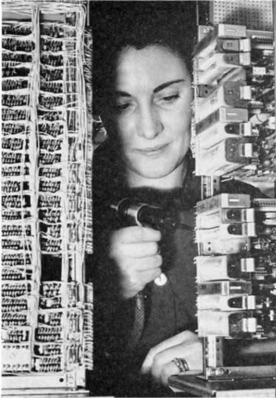
Wire wrapping with the aid of a pneumatic gun on a platine, integral part of a crossbar multistage switch.
