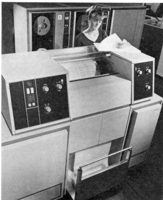
The line printer unit, part of the peripheral equipment. It has its own control unit and maintenance takes only ten minutes a day.
