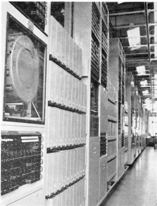
A suite of register translators in the Tower Exchange. The RT in the foreground has had a panel removed to show the position of the magnetic drum which is located under the circular cover.
