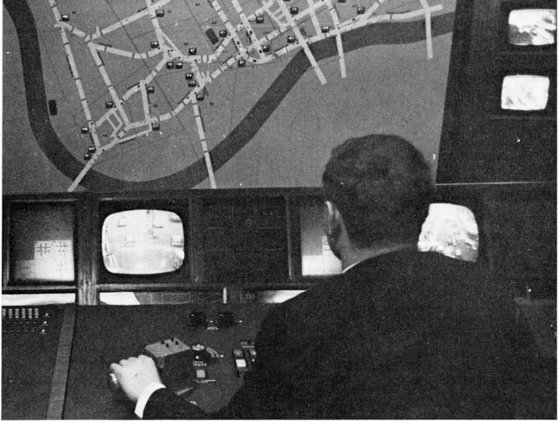
A Police Sergeant at Scotland Yard's new traffic control centre watches the build up of traffic on the television screens. He controls the eight television cameras with the box in his left hand.
