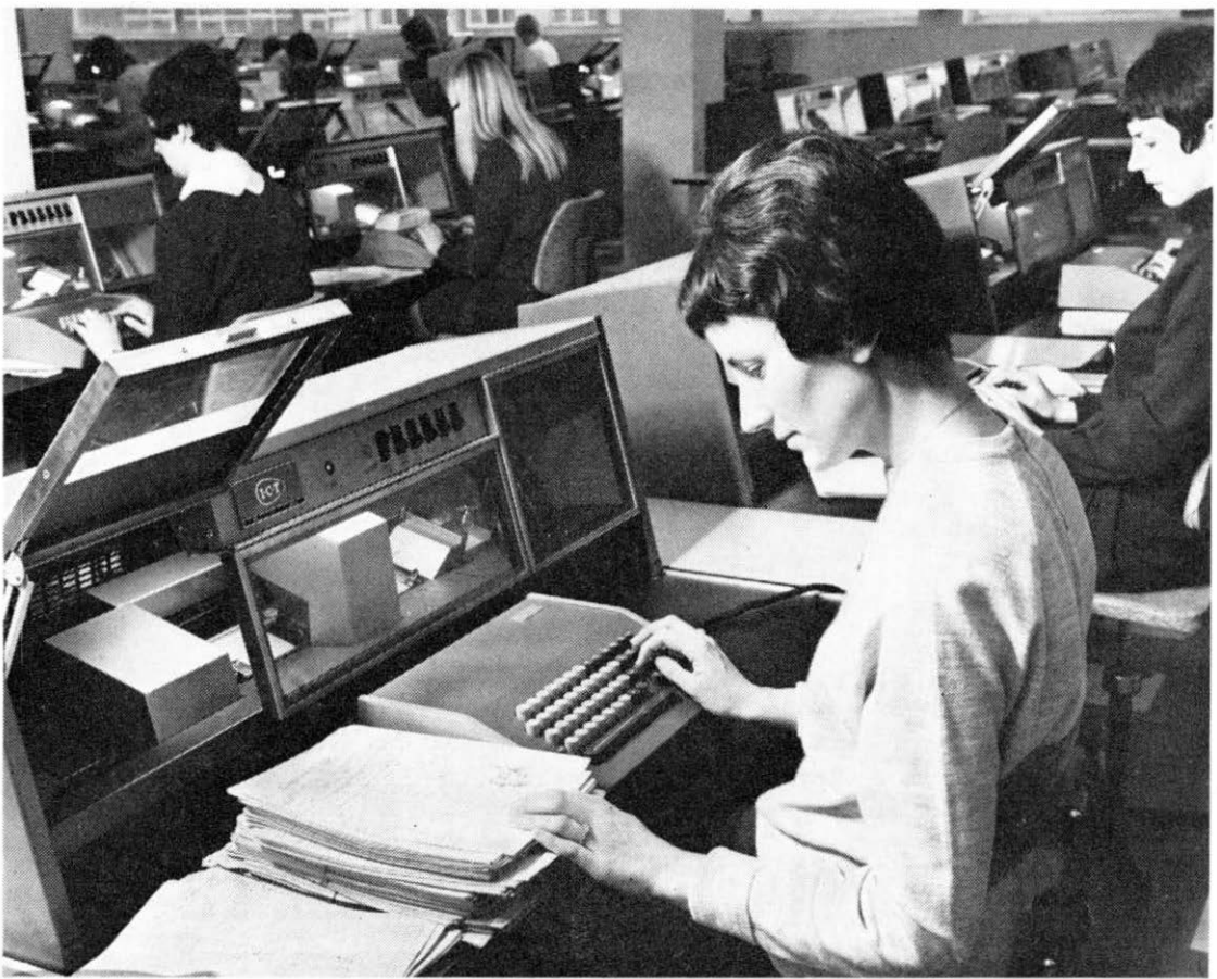
At the Portsmouth Computer Centre, where the processing is being carried out, Machine Operator Miss S. J. Quarrington punches the information from tally cards into 80-column punched cards.
