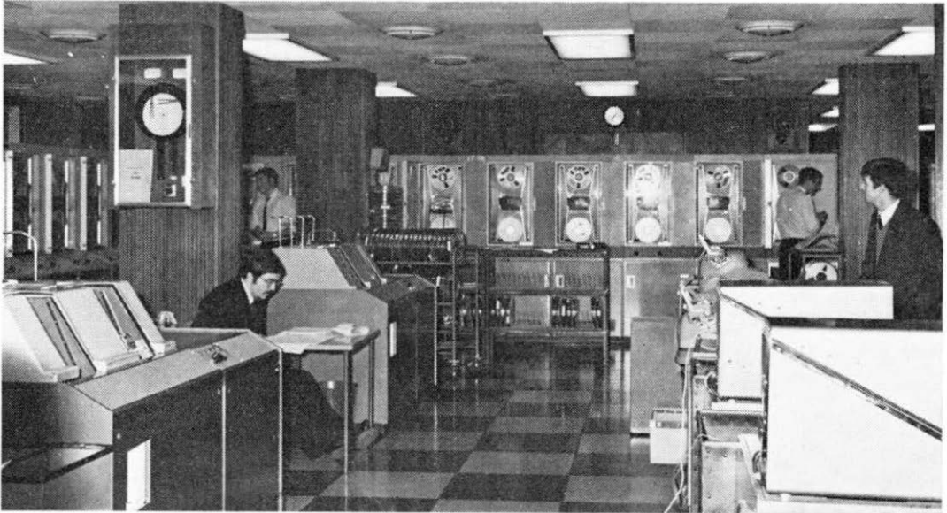
Information from punched cards is transferred to magnetic tape in the Charles House computer room.
