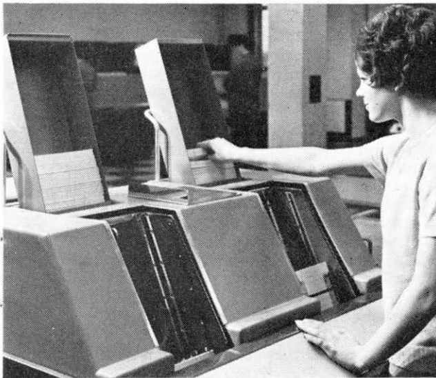
Machine Operator Miss C. M. Chittleburgh feeds 80-column cards into the computer's card reader which can handle up to 600 cards a minute.
