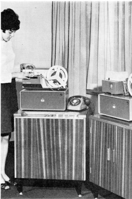
An operator feeds punched tape into the tape reader of a modern data terminal equipment for use with Datel 600 automatic answering facilities. The left-hand cabinet houses the controls, error-correcting and control circuitry.
