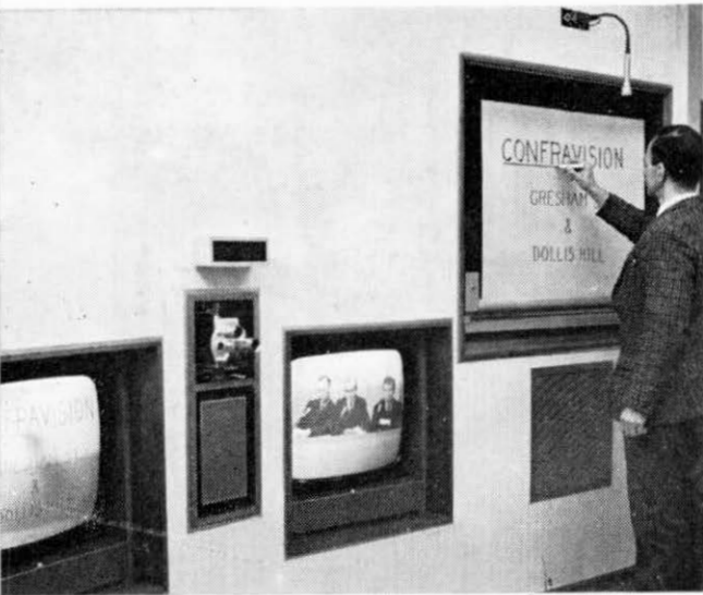
Below: A front view of the studio equipment cabinet. Sound, vision and lighting circuits are controlled from this cabinet by way of the control box in the studio
