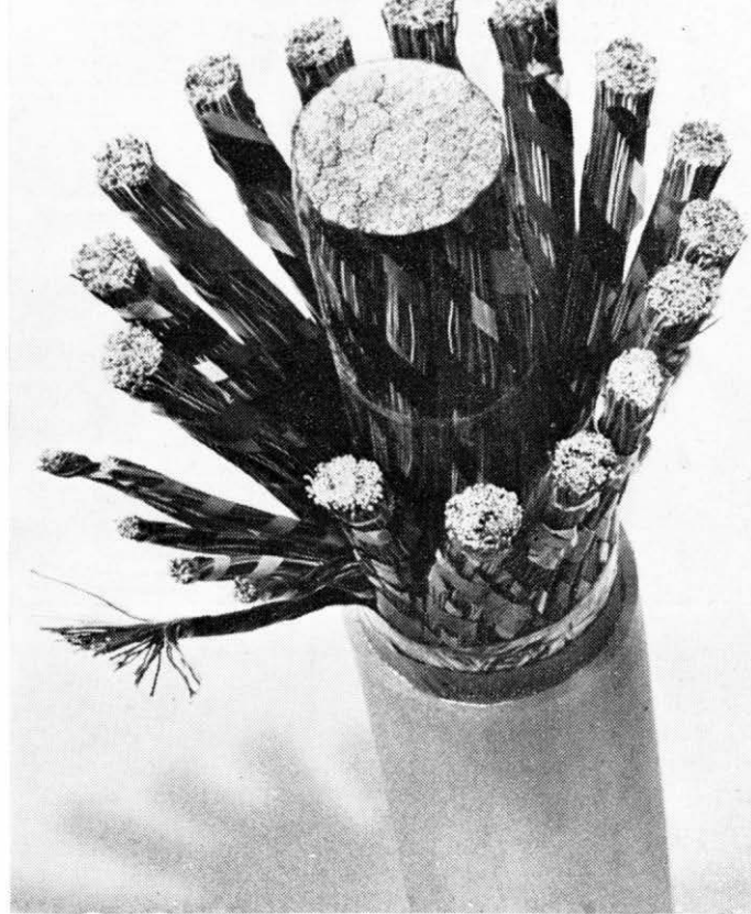
Above: A cross-section of the new cable. Each wire of the 4,800 pairs can be identified by means of a coloured code and each unit by coloured tapes surrounding the units.
