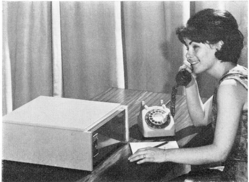
A Post Office photographic assistant poses with a Datel Modem No. 1 which can cater for automatic answering facilities.
