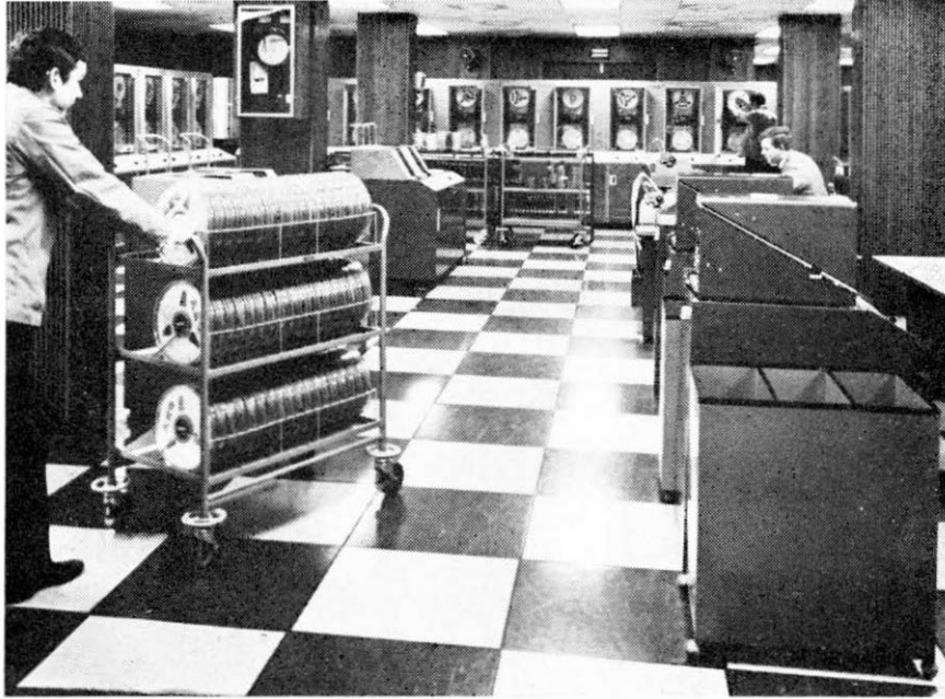
Left: One of the three LEO 326 computers in London, now being used for telephone billing and a wide range of other work
