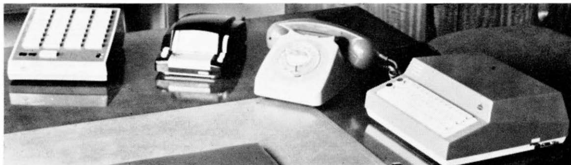
The range of repertory diallers. Left to right: the Autodial No. 101A, which stores up to 32 numbers; the Magicall, which stores up to 400 numbers on a magnetic tape; the telephone No. 746 required with any repertory dialler; and the Autodial No. 102A, storing up to 30 numbers.
