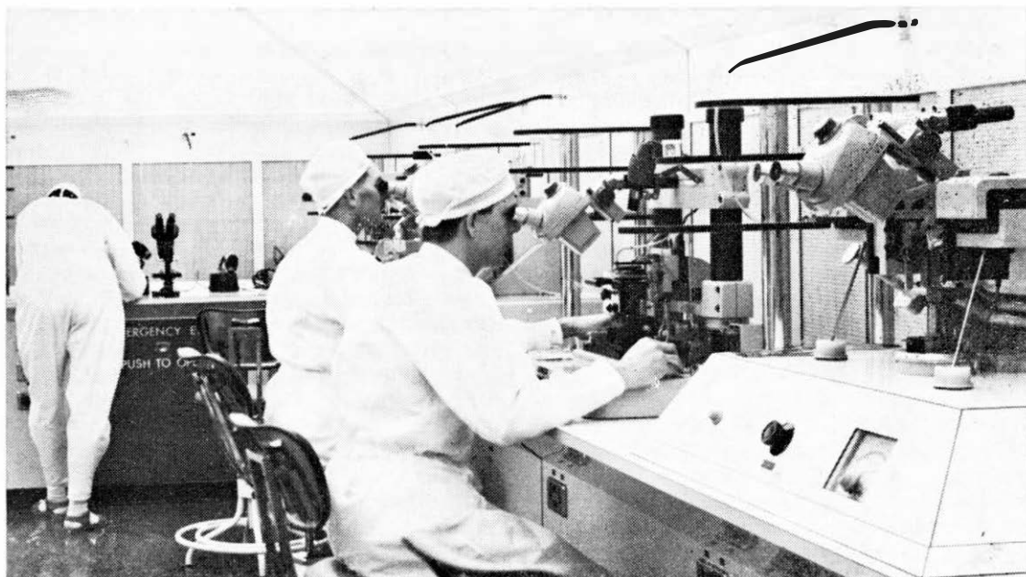
Operators at work in the special clean room where the air is continuously filtered.
