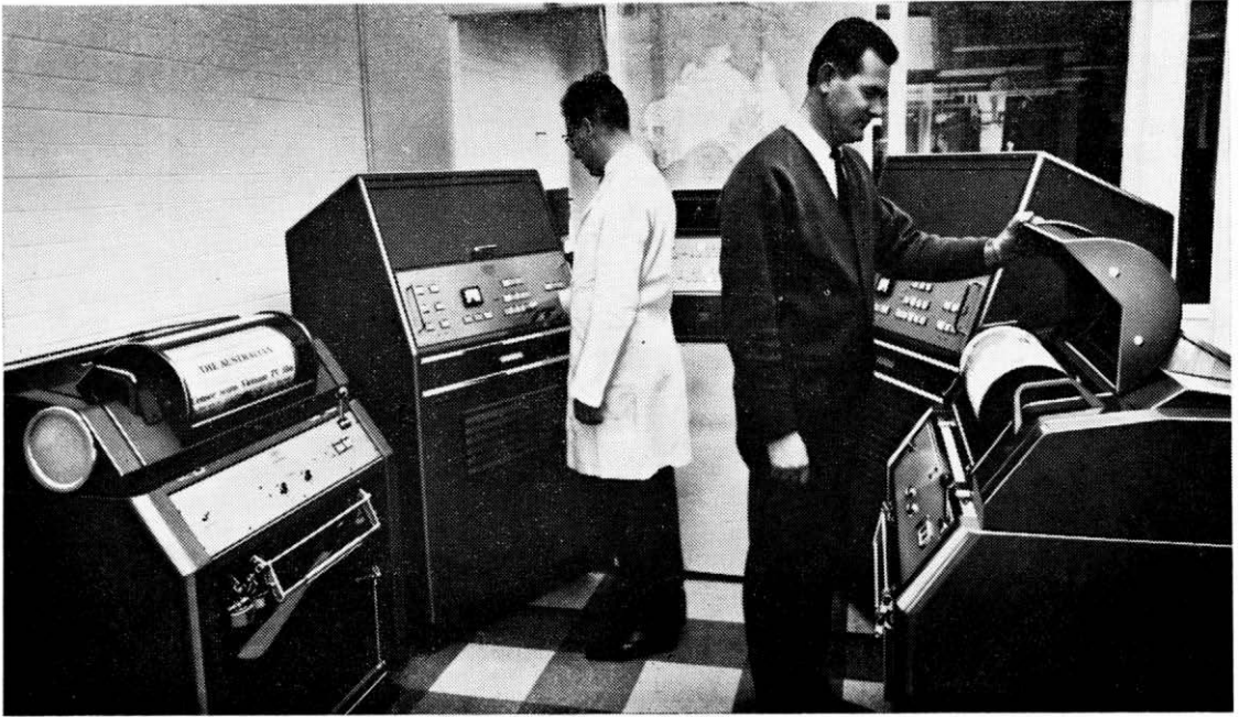
The facsimile control room of the Australian. The transmitter (left), receiver (right) and electronic consoles are similar to those used by British newspapers for high-speed facsimile transmission.
