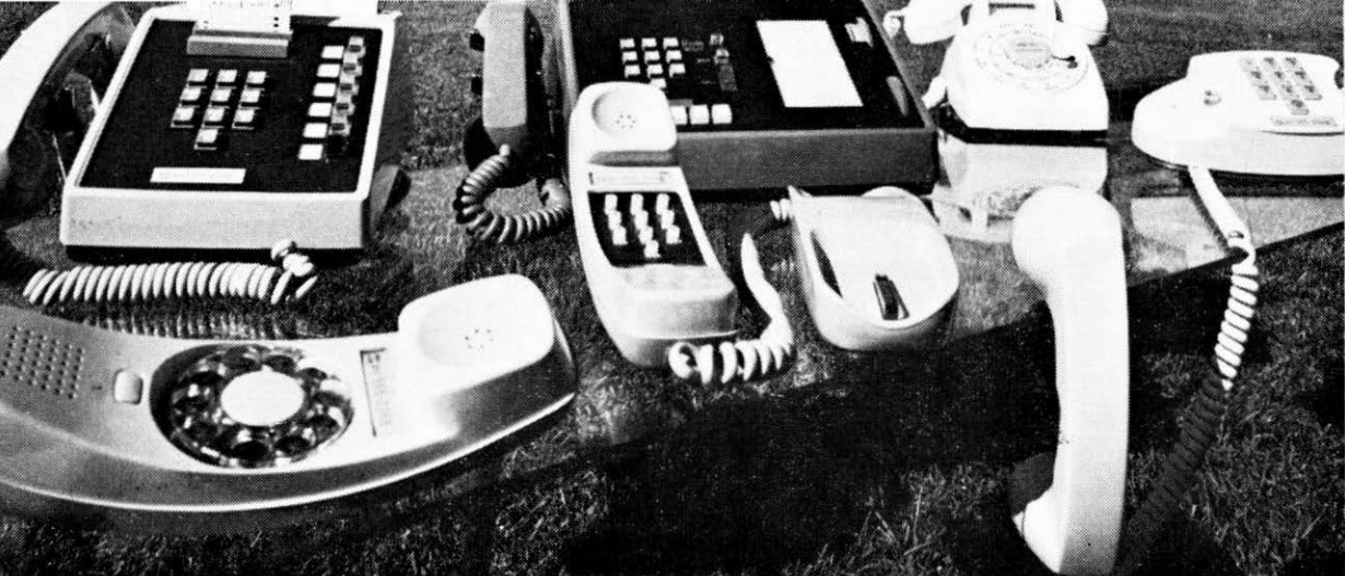
Six Bell telephones. Front: two Trimline telephones. Rear (left to right): the Card Dialler, the Call-a-matic, the 500 set and the Princess telephone.
