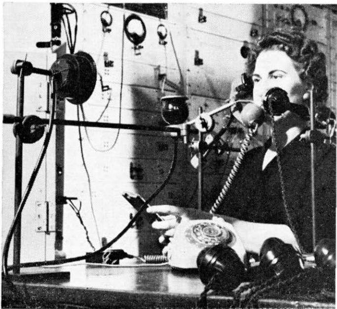
Miss Yvonne Gordon, of the Speech Test crew, takes part in a sound articulation comparison of different telephone instruments.
