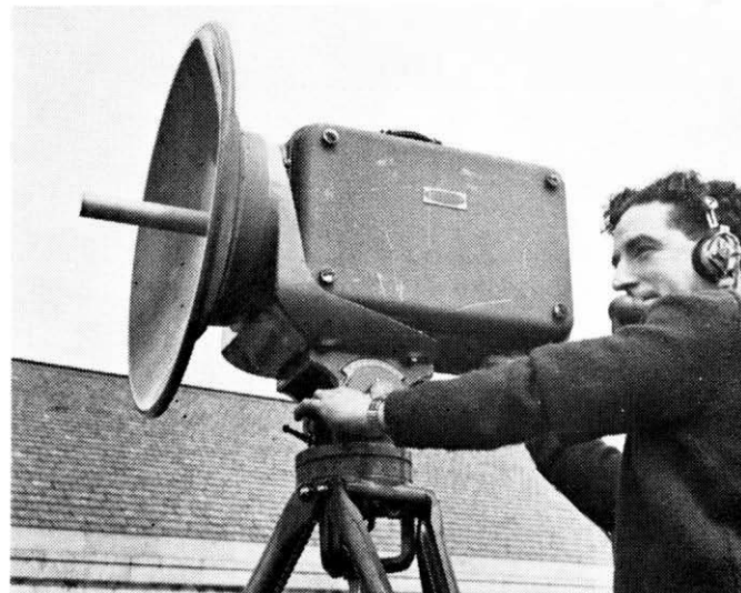
Technician 11A Mr. J. T. French, of the London team, lines up an 11 Gc/s two-foot aerial. The aerial is connected to the terminal equipment by up to 300 feet of coaxial cable.
