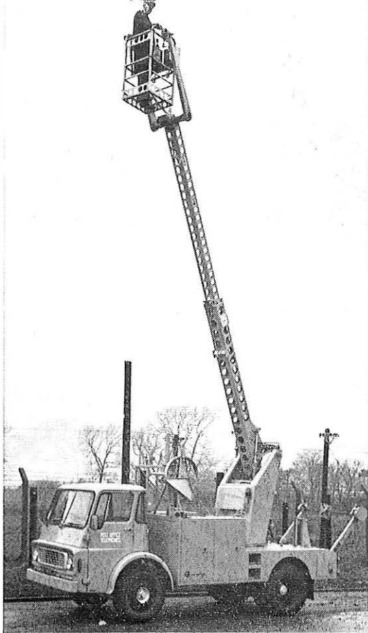
Telsta's telescopic boom reaches 36 feet high. In the metal basket is AEE Mr. G. V. Hunt.
