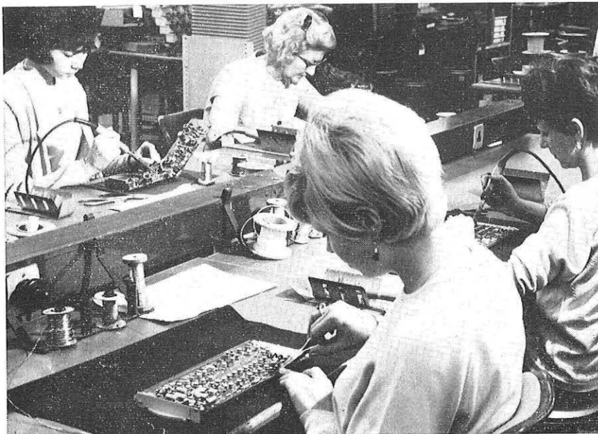
Girls at STC's Basildon factory assemble units for PCM terminals. The Post Office has already decided to order £6 m. worth of PCM transmission equipment.
