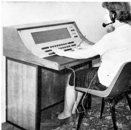
The GEC PABX 4 follows the conventional cordless switchboard design and is made in light teak to blend with modern office furnishings.
