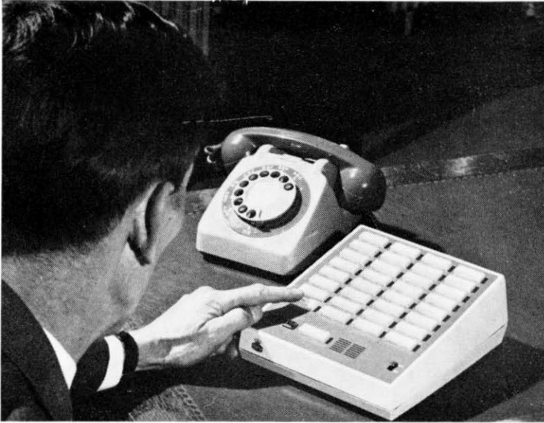
The Key Callmaker provides 32 telephone numbers which are selected by individual press buttons. A small loudspeaker is also incorporated in this design for monitoring the progress of the call.
