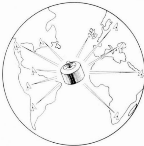
Left: Diagram shows how an Intelsat III satellite—three of which are due to be launched in 1968—will provide communication between many earth stations simultaneously.
