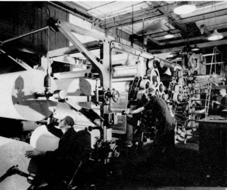
Left: One of the HMSO rotary printing machines on which telephone directories are produced. Below: Completed directories roll off the Sheridan Gatherer and Binder.
