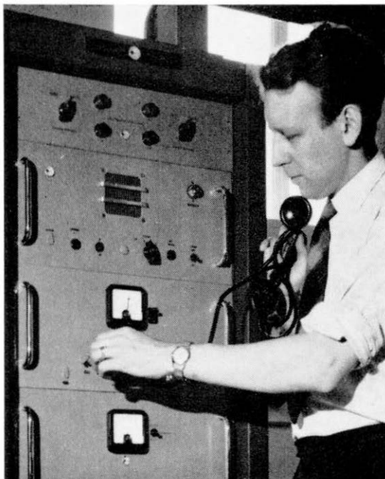
Above: Technical Officer Mr. J. Buss adjusts a VHF transmitter at the Fairseat microwave relay station, near Sevenoaks, Kent.
