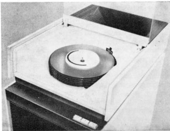
An exchangeable disc store. The pack of six discs can be replaced by the operator. The discs are 14 inches across and the pack weighs 10 lb. Picture: Courtesy International Computers and Tabulators.
