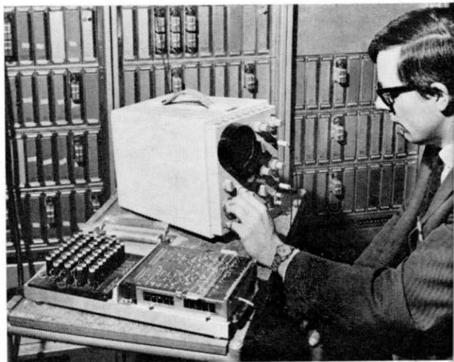
Assistant Executive Engineer P. T. Hercus checks the performance of one of the plug-in units of the new tdm equipment by means of a cathode-ray oscilloscope connected to a printed circuit.
