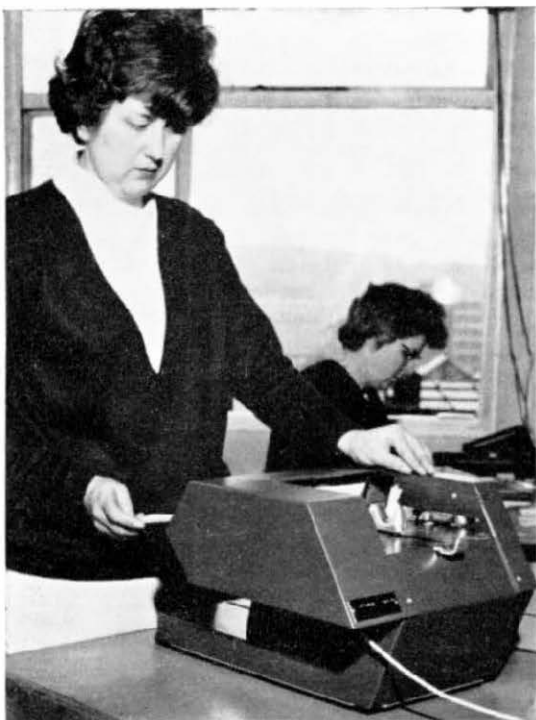
Left: Mrs. R. Willett, a telephonist at Brighton Telephone Exchange, holds the 1,000th ticket selected for her by the card counter. These machines are now being supplied to the largest switchboards to speed ticket counting and Trunk Call Analysis sampling.
