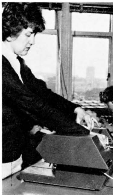
Mrs. Willett reloads the counter machine with another batch of trunk tickets. The machine can count tickets at the rate of 600 a minute.
