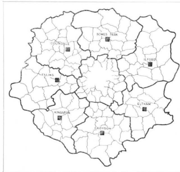
This diagram shows the future division of the director area for routing and switching purposes. The approximate locations of the proposed sector switching centres are also shown here.
