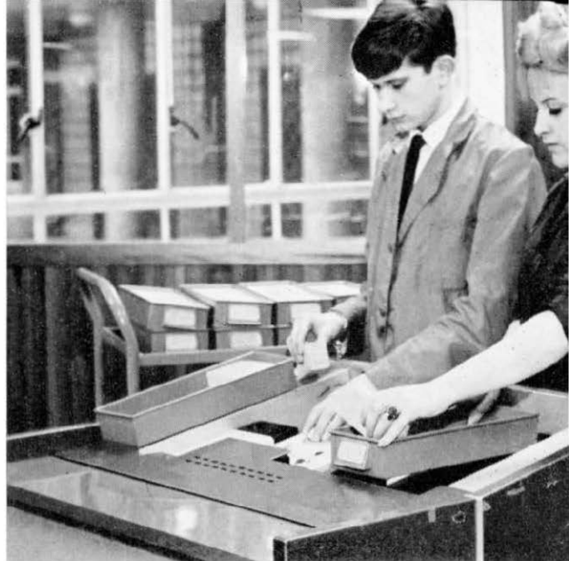
Millions of telephone bills are now being produced by computer at the London Computer Centre. Here, a 40-column card-reader for MATS cards is being used.
