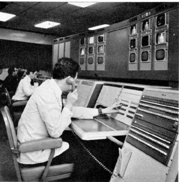
Left (top): A close-up of the vision test console, showing an Engineer connecting a vision circuit to a picture monitor by press-button. In the foreground is the keyboard through which communication is made with other stations.
