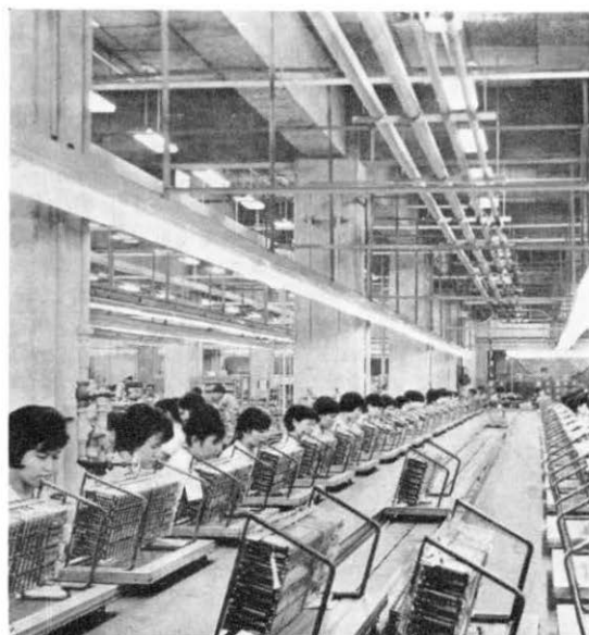
Left: A busy scene in the crossbar switch assembly room of a NTT factory. Above: Operators at work on cordless switchboards in Tokyo's international telephone exchange.
