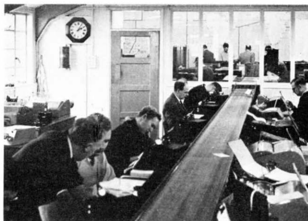
Left: A radio officer on board the Shell tanker Serenia sends a Morse message to Burnham for onward transmission to the Shell Centre in London. Above: The teleprinter room at Burnham from where circuits connect to the inland telegraph network and also to telex subscribers, Lloyds, the Admiralty and the Meteorological Office.
