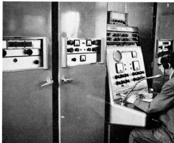
Above: An operator at work on the console controlling the single-sideband radio-telephone circuits between Humber Radio station and oil rigs. Similar equipment has been installed at Stonehaven and Cullercoats radio stations. Drilling rigs also have conventional ships' radio-telephone equipment for communicating with coast stations on normal shipping frequencies.
