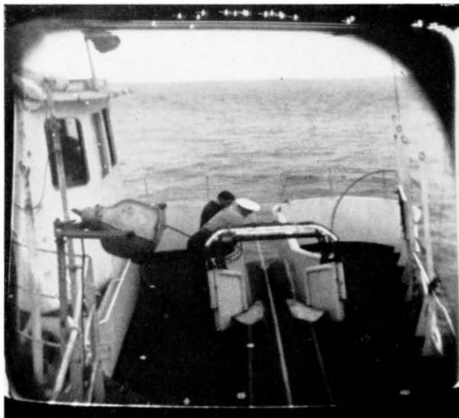
These two pictures show how operators on the closed-circuit television screens saw the test cable running astern (right) and (above) Monarch's centre-castle tank bell mouth through which cable enters and leaves the tank.
