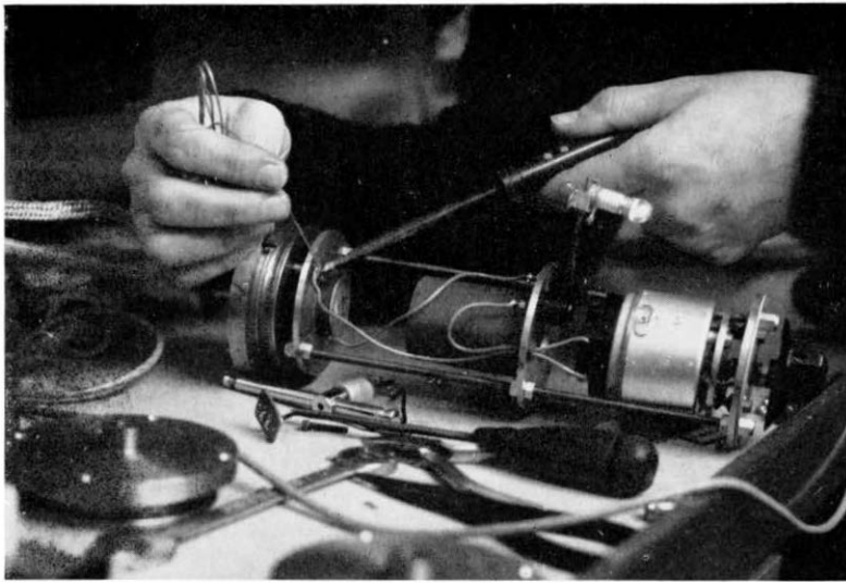
An engineer at the Post Office Research Branch at Dollis Hill, which also took part in the Monarch trials, at work on a time-bomb. Note the clockwork mechanism on the right.
