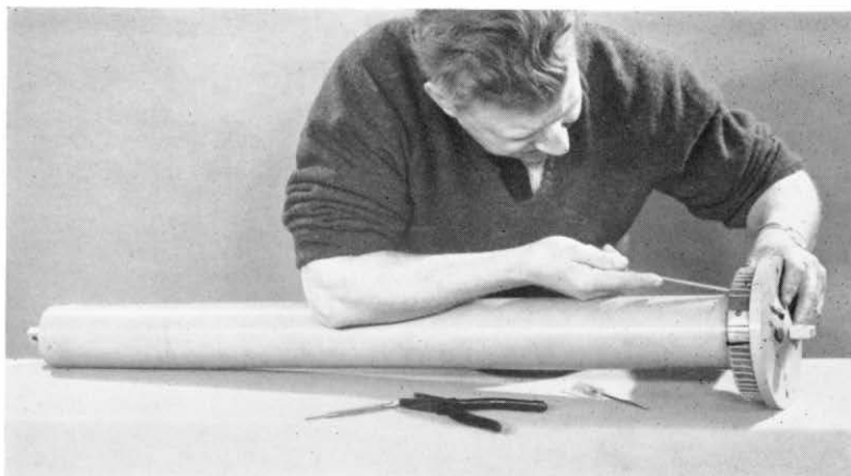
An engineer puts the final touches to the base-plate of a sonar beacon, or "pinger," containing the transmitting equipment, before it is lowered to the sea-bed.
