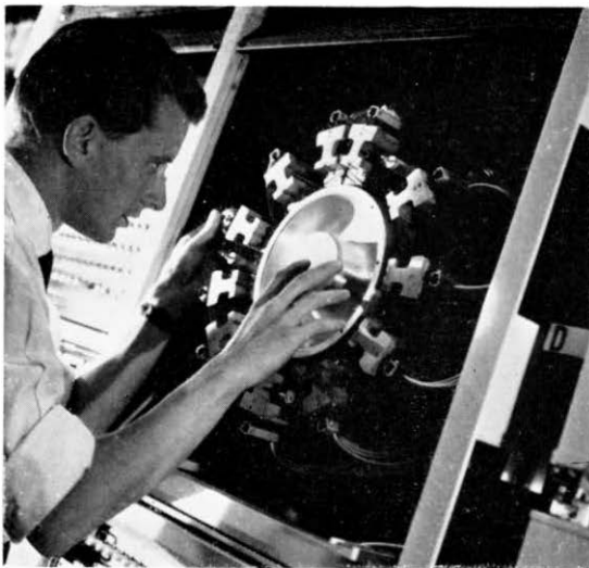
Above: Mr. R. Hall, a contractor's engineer, assembles a magnetic drum register translator for routing calls to the provinces.
