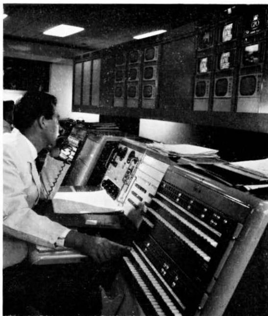
Above: Mr. R. Hall, a contractor's engineer, assembles a magnetic drum register translator for routing calls to the provinces.
