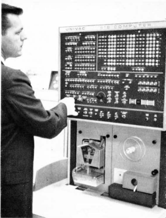
(Left) The control panel of a Univac 418 computer at Goddard. (Above) Information from the computer memory store is read out on high-speed printing equipment during tests at the Goddard Space Flight Centre. Similar equipment will be installed at the London centre.
