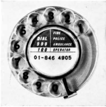
The all-figure dial (above) which all new telephones will have after the change-over is completed. On the right is a selection of all-figure dials used in Australia (top left); Egypt (top right); Singapore and Hong Kong (bottom left) and in Russia (bottom right).
