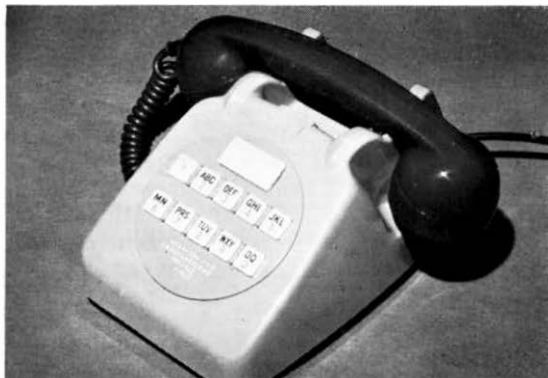
Experimental press-button telephone (the final version will not necessarily look like this) to be introduced soon.
