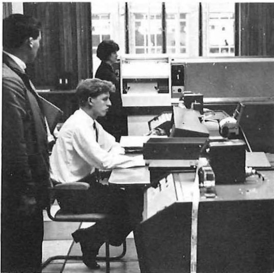
This picture shows the paper tape readers (foreground), the console and the Anelex printer at the Charles House centre.
