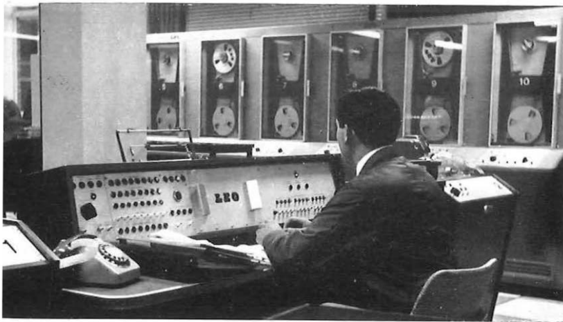
This picture shows the paper tape readers (foreground), the console and the Anelex printer at the Charles House centre.
