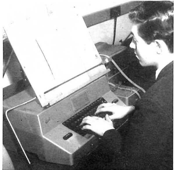
Below: Machine operator T. J. McEvoy punches out a programme for the Dollis Hill computer on an autocode machine.
