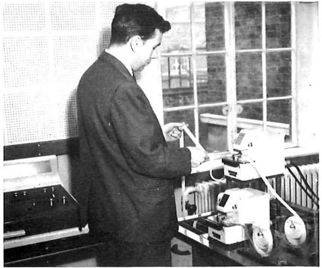
Mr. P. Strawson, senior machine operator, checks tapes as they pass through the paper tape readers of the Dollis Hill computer.
