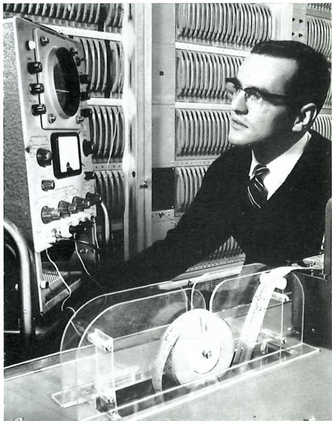
Systems testing of the electronics on a Leo 326 computer. The electronic racks (in background) receive the information input by the punched tape (in the foreground).
