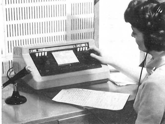
A recording console at the London multi-service installation. An operator selects the service before recording.
