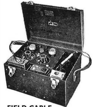
FIELD CABLE TEST SET For locating breaks or short-circuits in sheathed multiple conductor cables within a fraction of an inch.
