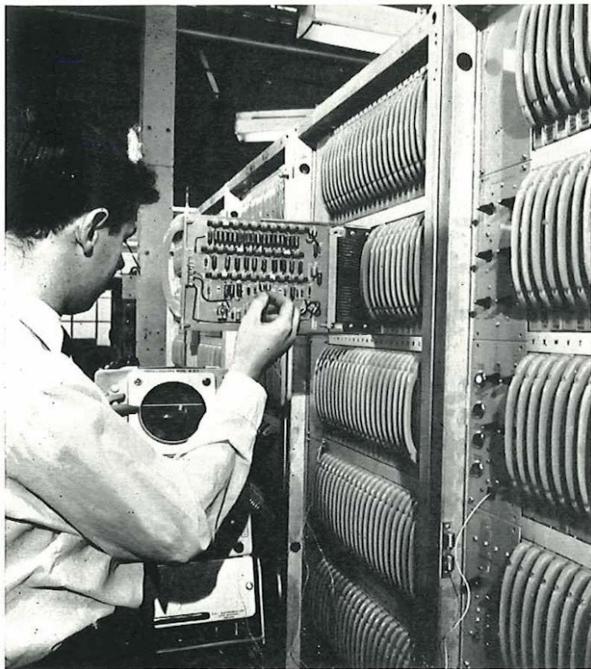
An engineer tests a logic circuit on the first LEO 326 computer ordered by the Post Office. The pictures illustrating this article are reproduced by courtesy of English Electric-Leo-Marconi.
