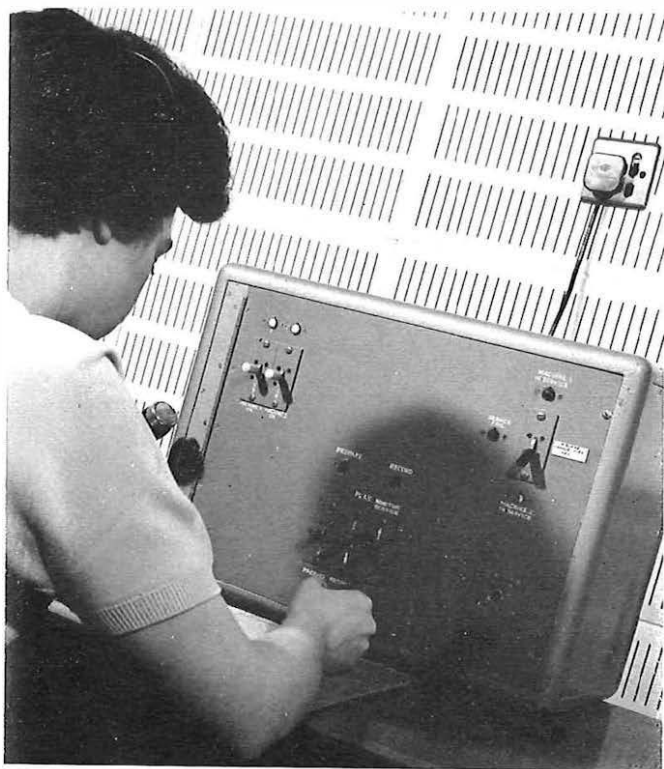
The console used for the Test Match Information Service to which are wired two machines, operating alternately. About 600 separate recordings are made each day during test matches.
