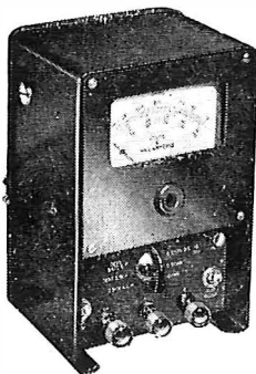
POST OFFICE TESTER A multi-range meter for testing subscriber apparatus and lines.
