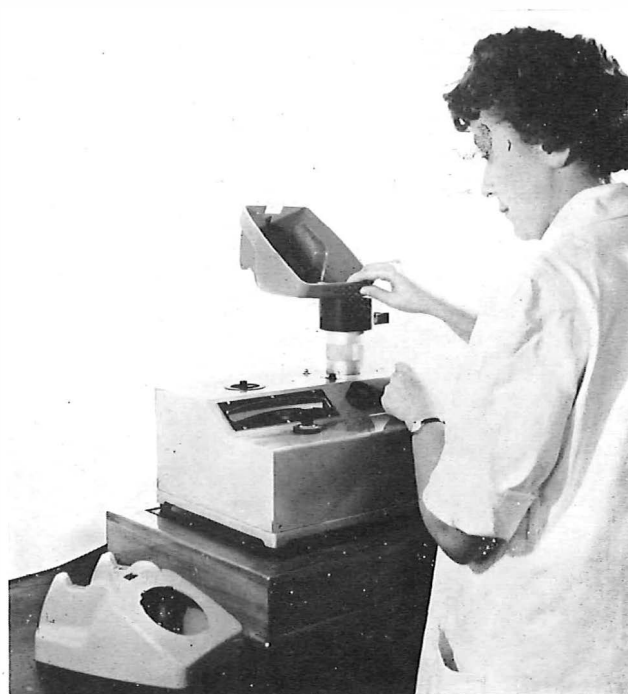
Mrs. M. Harridge, of the London Materials Section, uses a tristimulus colorimeter to measure the colour shade of a telephone case. The colorimeter defines colour in numerical terms.
