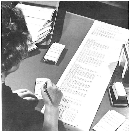
An operator counts the "MOM" signals to assess the chargeable time. The signal is generated every six seconds.
