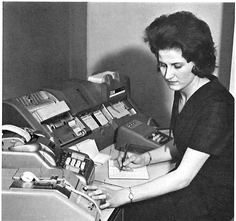
An operator at the Shell Data Process Centre supervising data tape to punched card conversation.
