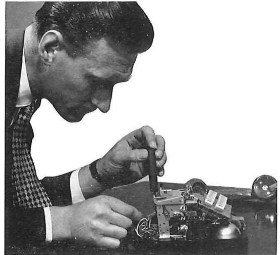
Above (top): Keying a number on a push-button telephone (seen alongside a dial telephone). The white rectangles above and below the keyset will contain the telephone number and brief instructions normally shown on the dial centre label. Below: a technician adjusts a push-button telephone from which the outer case is removed. Left: Diagram of a push-button telephone showing the arrangement of keys.
