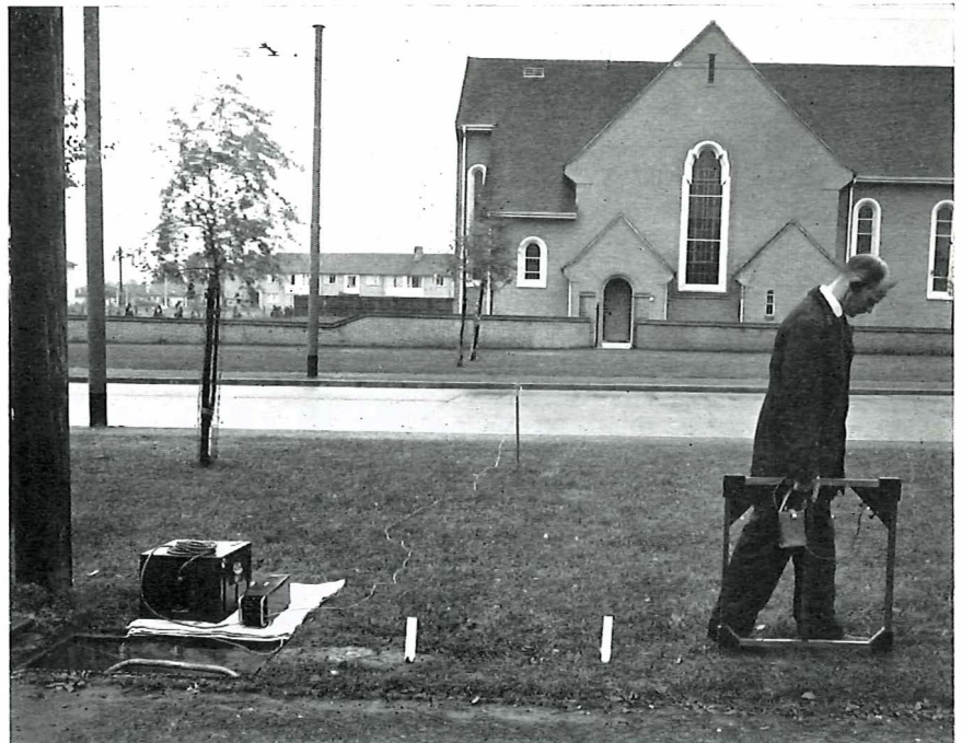
THE OLD. The same task is carried out with the obsolescent apparatus which includes a large and cumbersome search coil.
