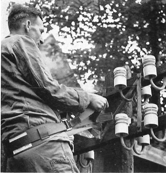
The new safety belt, showing how the adjuster works. The belt has a minimum breaking strength of 5,000 lb.
