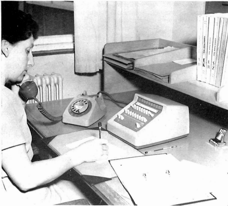
An operator with the PMBX No. 2/2A on which exchange calls can be held by operating a key, thus enabling her to speak to an extension without being overheard by the caller.
