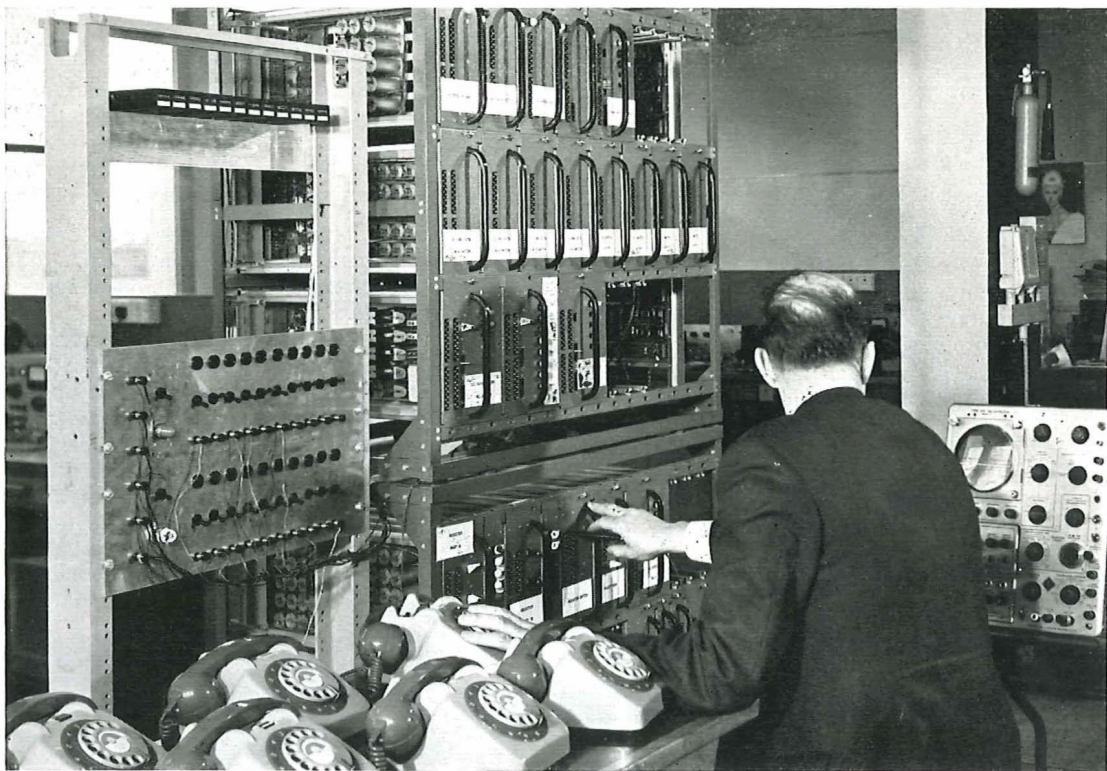
An engineer at work on a laboratory model of a space-division exchange.
