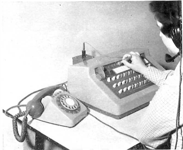
Above: A PMBX 2/4A for use at the Jewish Blind Society, fitted with a converter to give an audible signal in the earphone when the probe is over the illuminated lamp. Below: A view of the magnetic bracket and probe when in the resting position.
