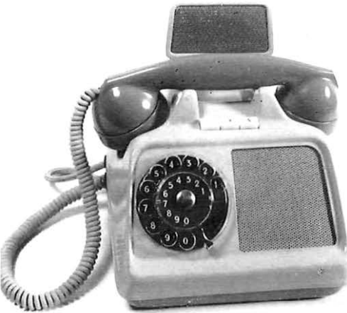
Above (top): The GEC single-cabinet type of LST, completely self-contained. A version of this model was adapted for use as the Post Office LST No. 2. (Centre): The ST and C voice-switched instrument; and (below): The Swedish WeGe voice-switched set. In a more recent model the loudspeaker is incorporated in the front of the instrument.
