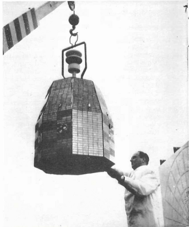
Relay II is examined by a technician at Cape Kennedy, Florida, before being launched. Relay II has over 8,000 solar cells.
