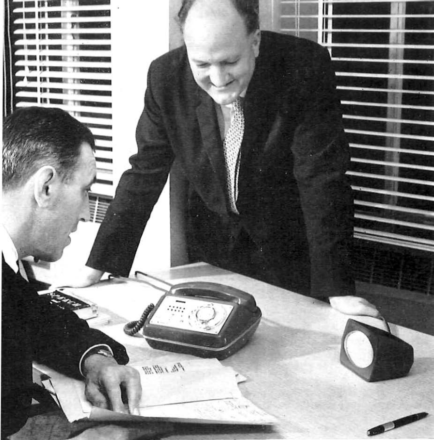
The author (left) and a colleague take part in a "group" conversation using the American A.E. Company's Speaker-phone. This set is partly voice-switched and will operate from line current. A flashing neon lamp in the press button provides a novel way of indicating when the set is in use.
