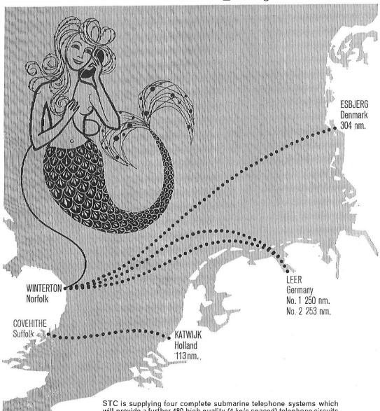
STC is supplying four complete submarine telephone systems which will provide a further 480 high quality (4 kc/s spaced) telephone circuits between the UK and the European Continent—a total of 920 nautical miles of cable, 81 submerged repeaters, 6 submerged equalizers, power feeding equipment and special terminal equipment. More than 700 n.m. of STC submarine cable and 56 STC submerged
