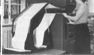
Two pictures of the Post Office's own LEAPS computer system. Left: An operator prepares data in punched tape form for input to the computer. Right: Payroll documents for issue to local pay units being printed by one of the two high-speed Samastronic printers. The printhead shown here is driven electrically from magnetic film on which payroll details have been recorded by the computer.
