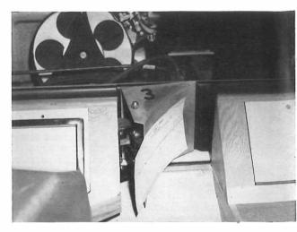
Telegrams travel along a V-trough conveyor and are diverted to transmitting positions by diverters working automatically on a timed cycle. This picture shows the automatic diverter in the operated position.
