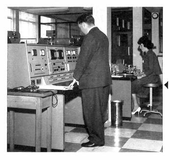
Technically, computer systems consist of a good deal of electronic equipment and devices assembled into complex logical structures coupled to many forms of high-speed electro-mechanical equipment —all operating usually in an air-conditioned room. Thus there are many technical features which must be taken into account when comparing the merits of different designs and long-term reliability and maintenance aspects are important factors.
