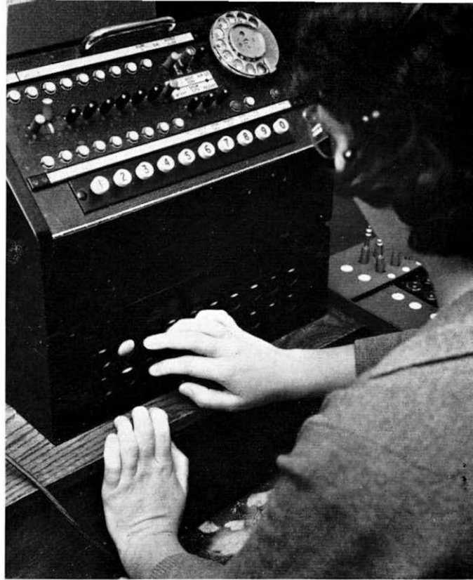
A PABX I standing on a doll's-eye plinth. The plinth converts the lamp signals of the PABX switchboard into doll's-eye movements which the blind operator is able to feel.
