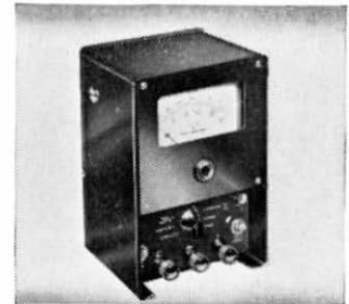
The Post Office Tester is a multi-range meter used for making tests on subscribers' apparatus and lines.
