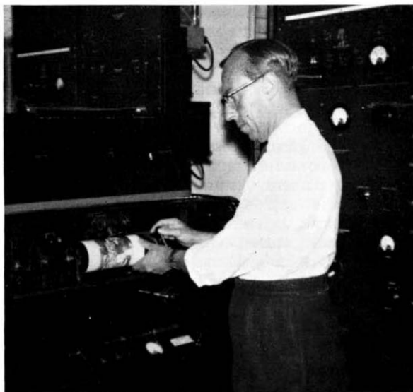
Technical Officer A. W. Kenison places the drum on the transmitting machine carriage before sending a picture to Australia.
