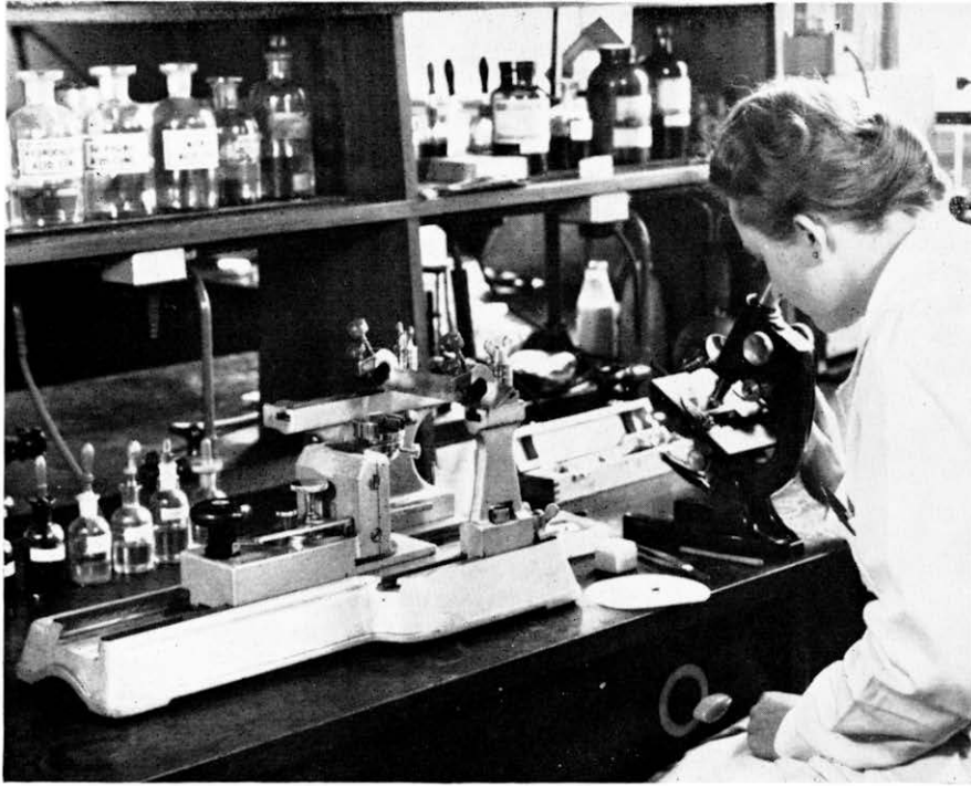
Miss Borroff examines a piece of wood for traces of decay. The microtome, on the left of the picture, enables thin sections of wood to be cut mechanically.
