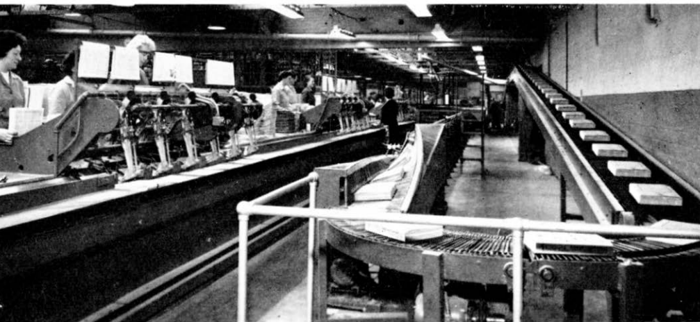
Part of the collating, binding and trimming machine at the Stationery Office printing works showing telephone directories being run off on a continuous belt.
