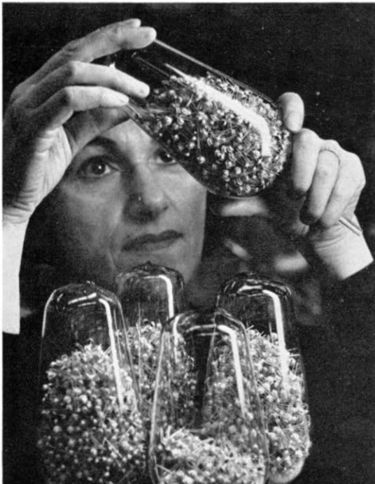
Left: Some of the transistors used in Telstar II . They were kept in vacuum jars to prevent moisture reaching them. Above: Showing how Telstar II will orbit the earth at twice the height of Telstar I .
