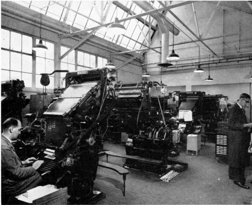
THE OLD Casting lines of metal type on an Intertype machine. Each machine has four magazines, each holding 90 matrices.
