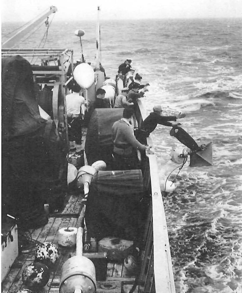
A dan buoy, with a radar reflecting top to mark the channel to be swept, is launched from the Royal Navy minesweeper Wolverton . From these buoys all navigation was calculated.
