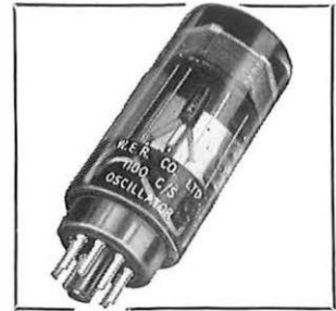
This fixed frequency oscillator is constructed on a standard octal base and encapsulated in epoxy resin.
