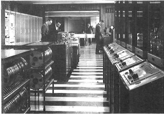
A general view of the LEO 111/1 installation at Hartree House showing the engineer's console and computer cabinets on the left, and magnetic tape units on the right. Courtesy: English Electric-Leo Computers Ltd.
