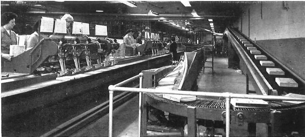
Part of the collating, binding and trimming machine at the Stationery Office printing works showing telephone directories being run off on a continuous belt.
