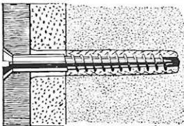
For screw fixings in solid materials Rawlplugs will take loads up to a million times their own weight. The tiny No. 3 ( $\frac{1}{8}$ ") is used for fixing cable clips, the largest No. 30 (1") for fixing electrical and other gear to walls or floors will take direct loads up to four tons.
