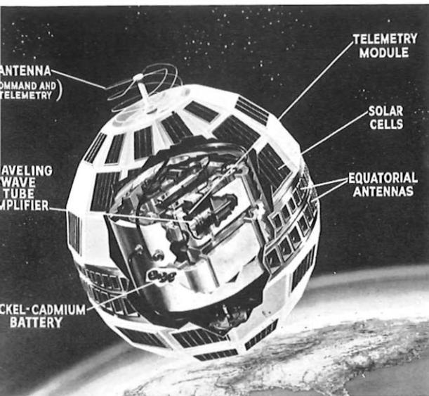
A cutaway drawing of *Telstar*. The decoder is immediately below the travelling wave tube amplifier.—*Courtesy: American Telephone and Telegraph Company.*
