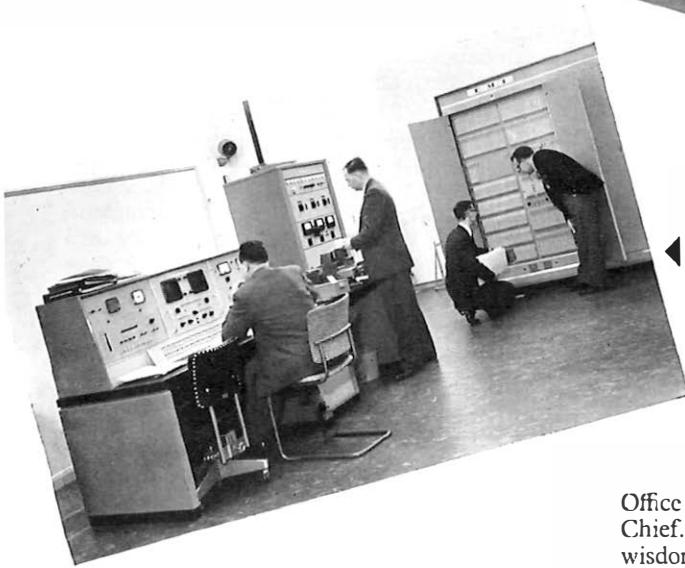
▶ The Ministry of Labour's Emidec 1100 computer installation at Watford. This machine is transistorised and British made.
