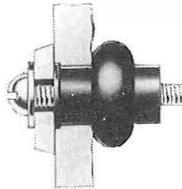
In the range of Rawplug Cavity Fixings the RAWLNUT has almost every advantage. It will make blind fixings in the thinnest of 'shell' materials, or in the larger sizes is suitable for hollow pot, or friable composition materials which will not hold conventional fixings. In situ it is vibration proof, waterproof, airtight, and insulative. It is extensively used in aircraft and car assemblies. There are sizes from  $\frac{1}{8}$ " BSW to  $\frac{3}{4}$ " BSW and alternative threads.
