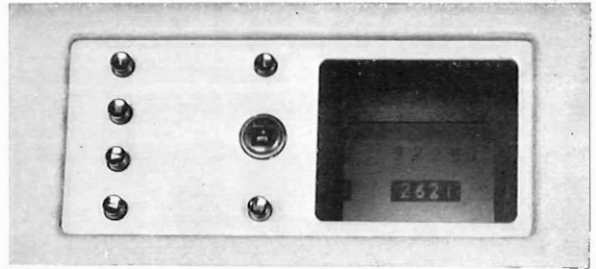
A close-up of the autoscope viewing panel. The meter reading appears at the top, with the subscriber's number below.
