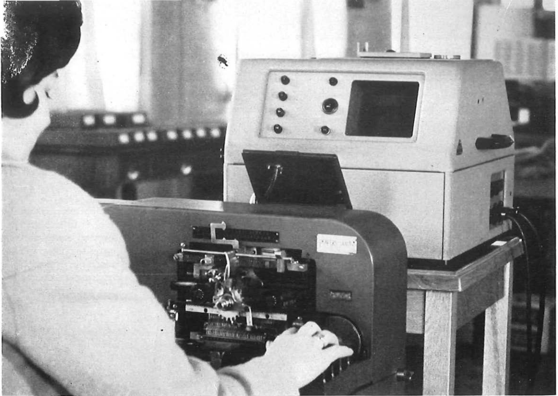
An operator punches the meter readings, displayed in the viewing panel of the autoscope in front of her, into cards.
