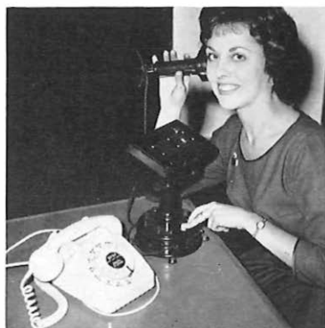
A visitor tries out an 1890 French Ader carbon and pencil transmitter telephone. Left is the latest telephone.
