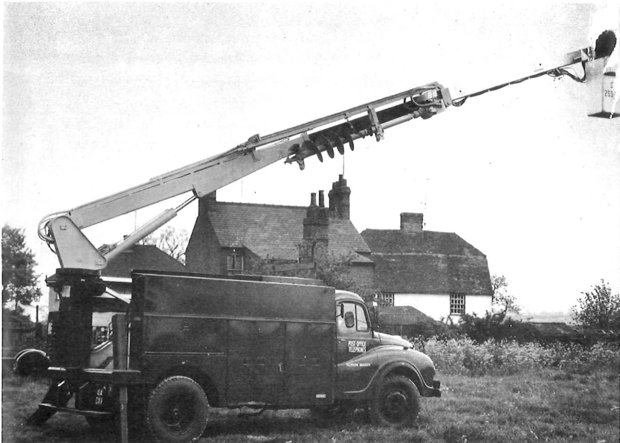
Perched in a bucket at the end of the derrick an operator demonstrates how he can raise himself aloft. The derrick can also be used for erecting new poles and lifting out old ones, handling stores and steering the pole hole borer.
