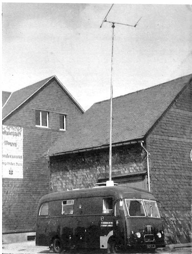
The Post Office mobile field-strength measuring van during its visit to Germany. The pneumatic telescope mast, 30ft high, simulates an aerial on a domestic chimney.
