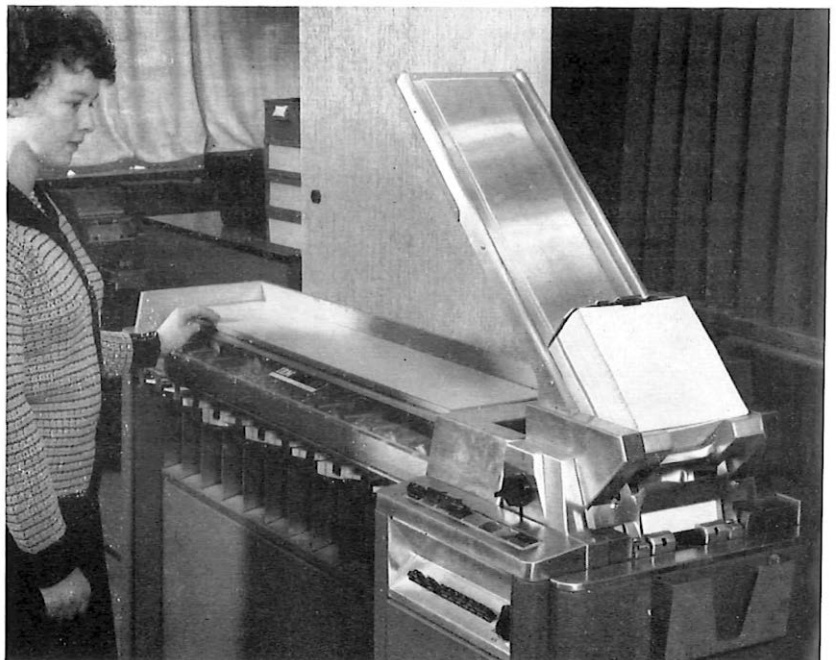
An automatic, high-speed machine of the type installed by the Post Office for sorting the telephone observation cards.
