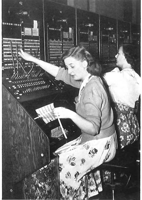
Teleprinter manual switchboards were installed in the CTO in the early 1940s. This system, adopted to save manpower, led to teleprinter automatic switching (TAS) now standard in Britain.
