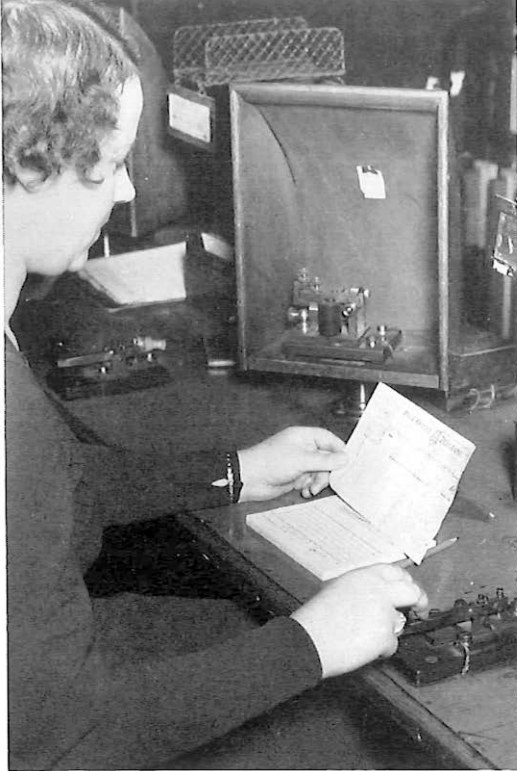
An operator at work on a Morse key and sound in 1934. This system was not popular because it gave many operators cramp.
